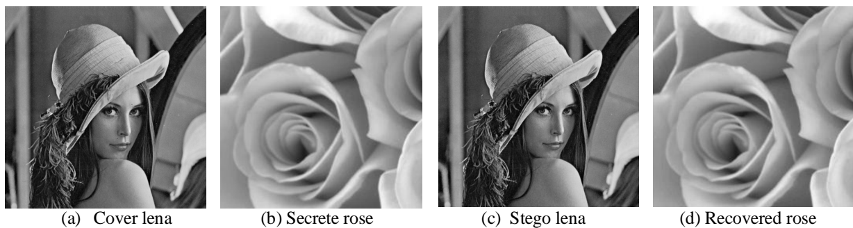
Fig. 5.6 (a) Original cover image ( 512 \times 512 ), (b) Original Secrete image ( 256 \times 256 ) (c) Stego image that has image (b) inside it, and (d) Recover image from (c)
