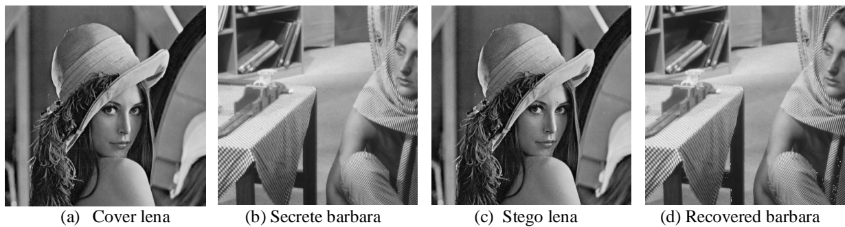
Fig. 5.10 (a) Original cover image ( 512 \times 512 ), (b) Original Secrete image ( 389 \times 389 ) (c) Stego image that has image (b) inside it, and (d) Recover image from (c)
