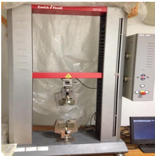
Figure 3.7: Tensile testing specimen (as per ASTM D638) and their testing arrangement
