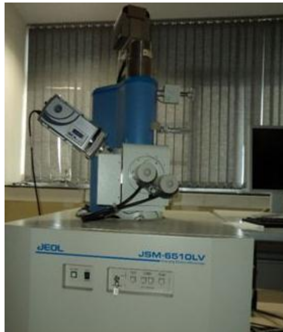
Figure 3.10: Scanning electron microscope (SAI Lab, Thapar University, Patiala)
