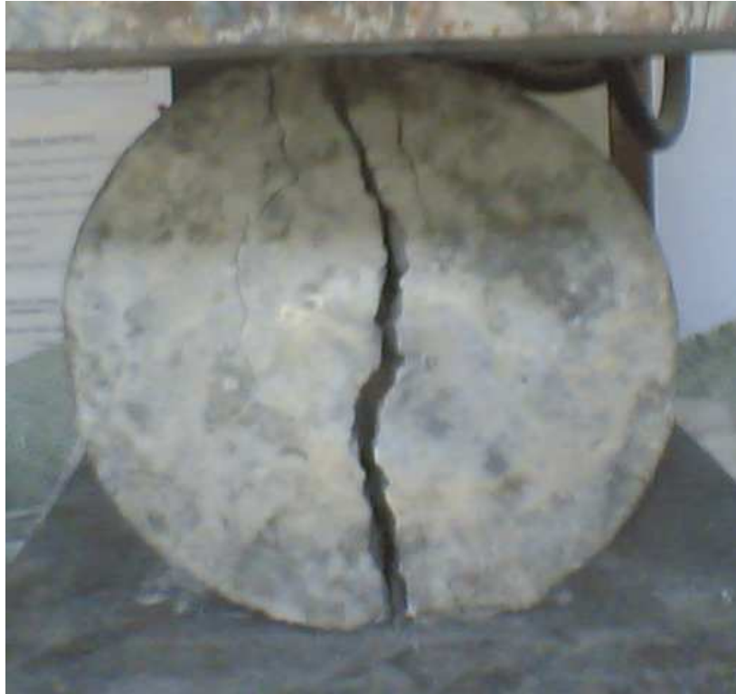
Picture-3: Splitting Tensile Failure of cylinder at various replacement levels of Foundry Sand
