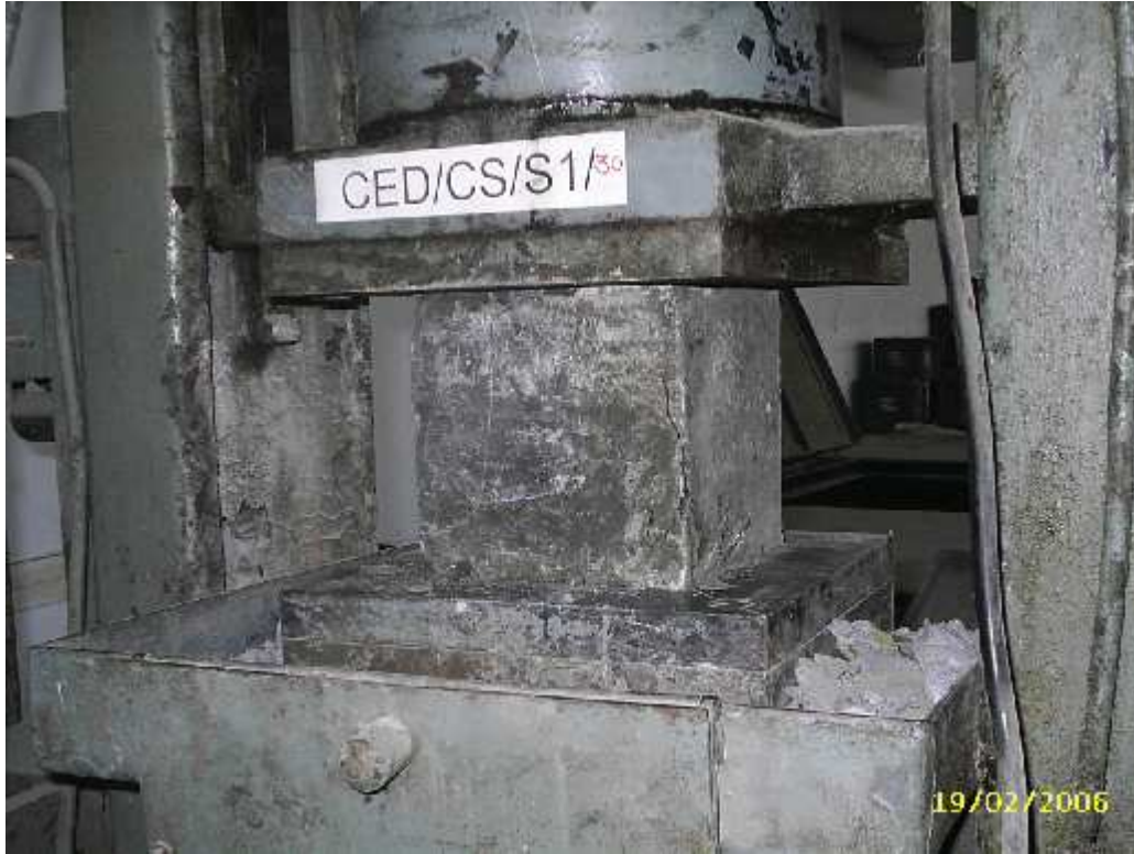
Picture-2 Compression Failure of cubes at various replacement levels of foundry sand
