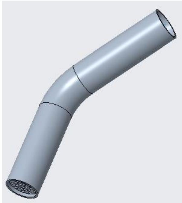
Figure 5.16 - Model of ATM 1 showing plate for blockage with holes at bottom
