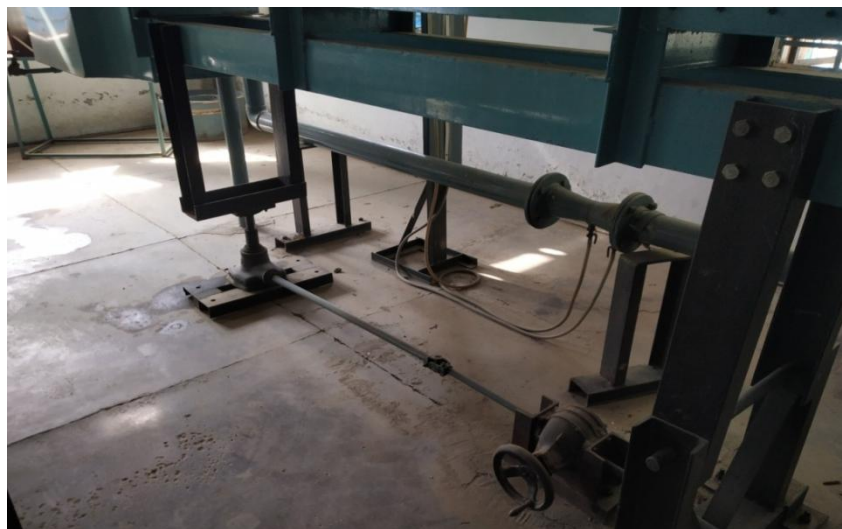
Figure 3.7 Hydraulic jack arrangement in the flume for changing slope
