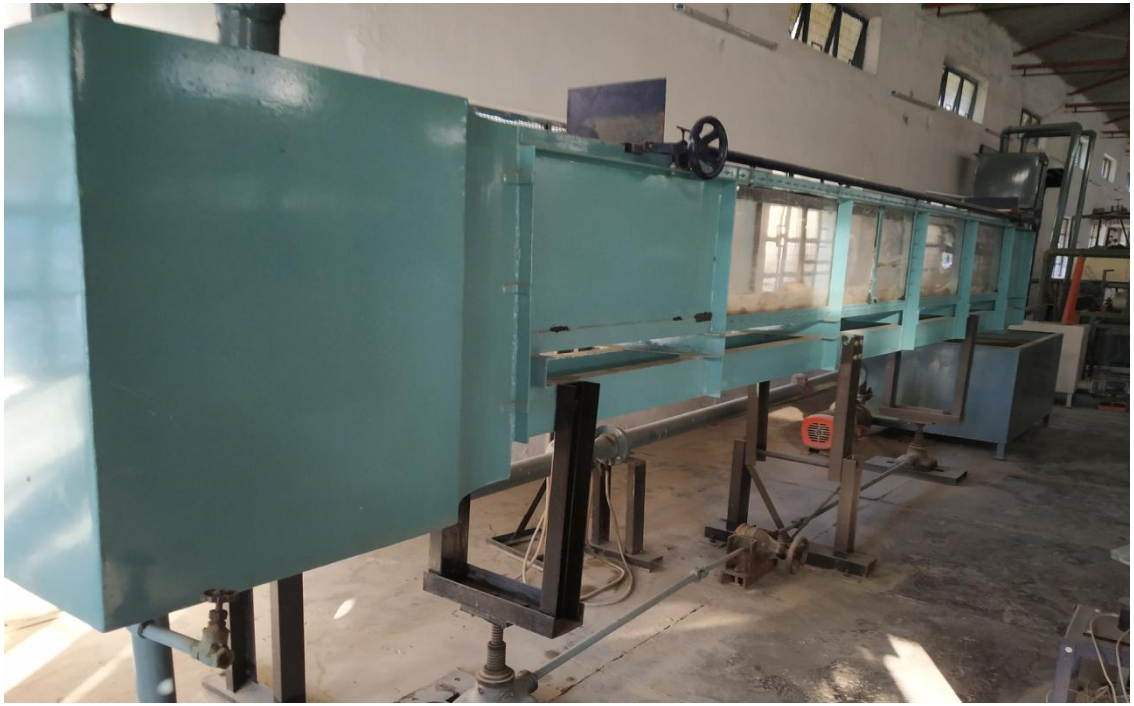
Figure 3.1 Tilting flume at Water Resources Lab, Thapar University, Patiala
