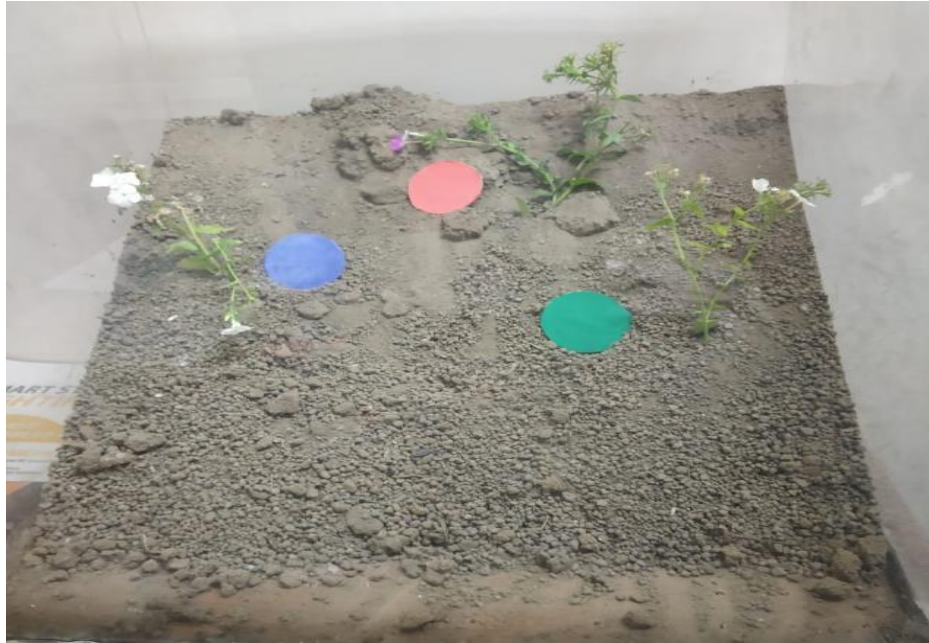
Figure 4.10: Placement of markers on slope
