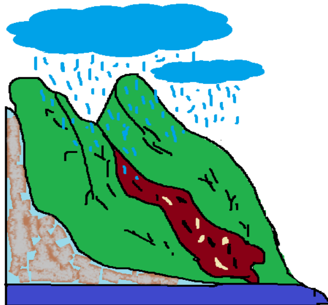
Figure 1.6: Debris flow landslide
