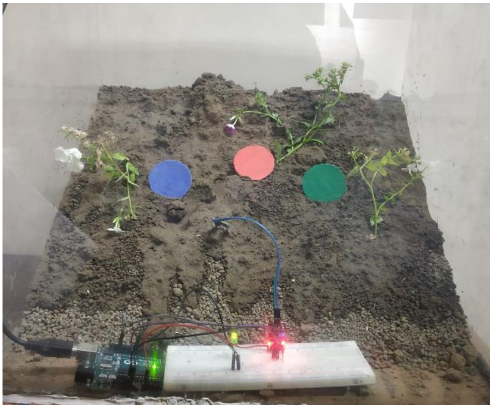
Figure 4.13: Generating an alarming signal that triggering landslide
