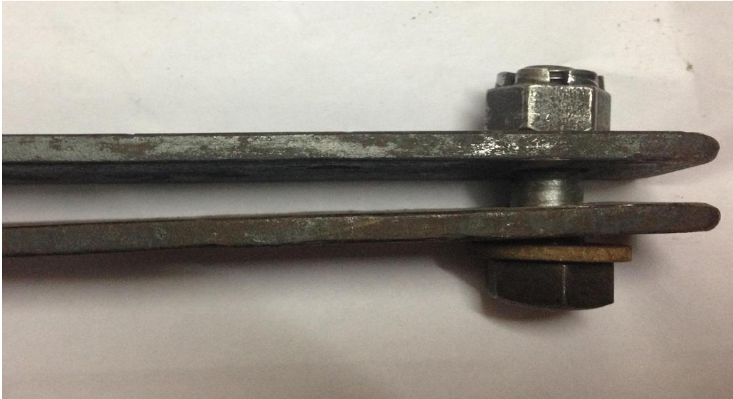
Fig: 4.13 Prepared fixture arrangement for Bearing Test
