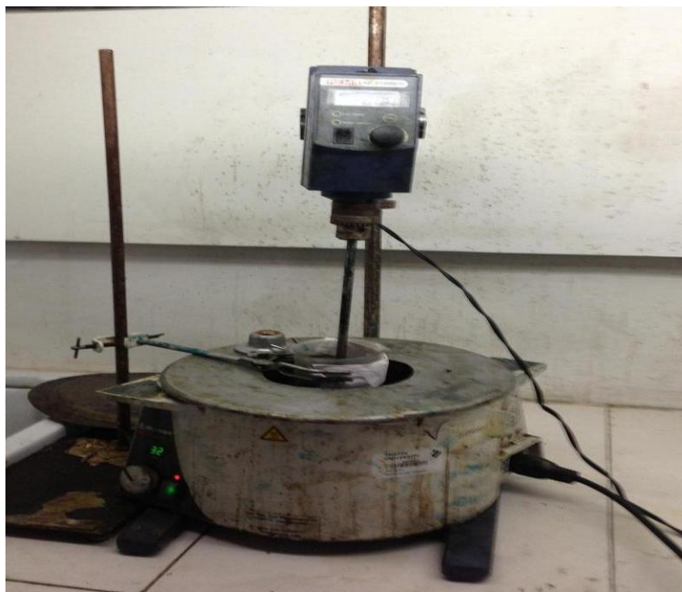
Fig: 4.4 Oil bath set-up with mechanical stirrer [Fluid Particle Mechanics Lab, Thapar University, Patiala]
