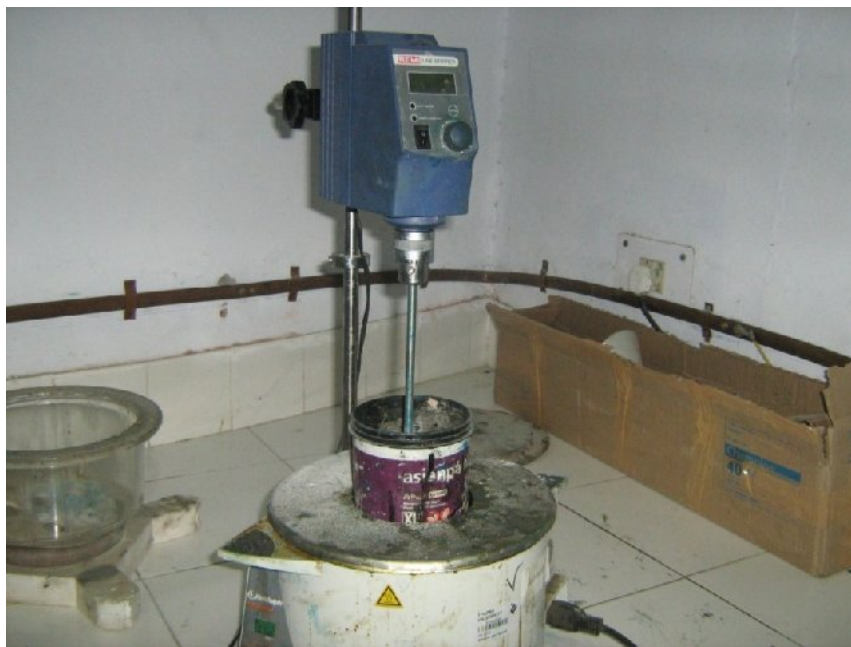
Fig. 4.4 Oil bath set-up with mechanical stirrer
