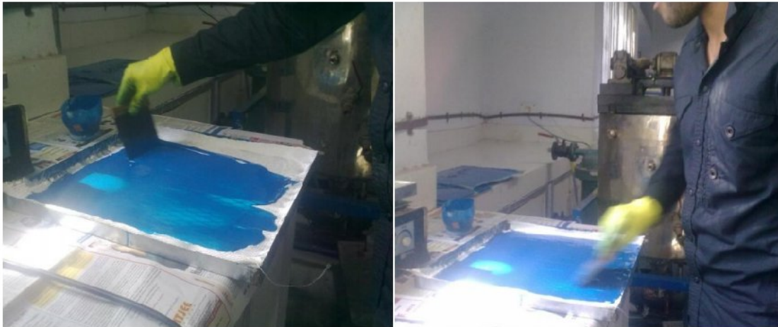
Fig. 4.7 Coating the glass fiber sheet with epoxy solution
