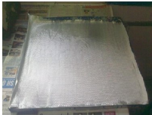
Fig. 4.3 Uncoated glass fiber mat used for making specimen
