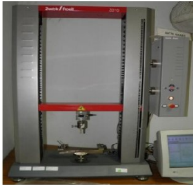
Fig. 4.16 Three point bend test machine
