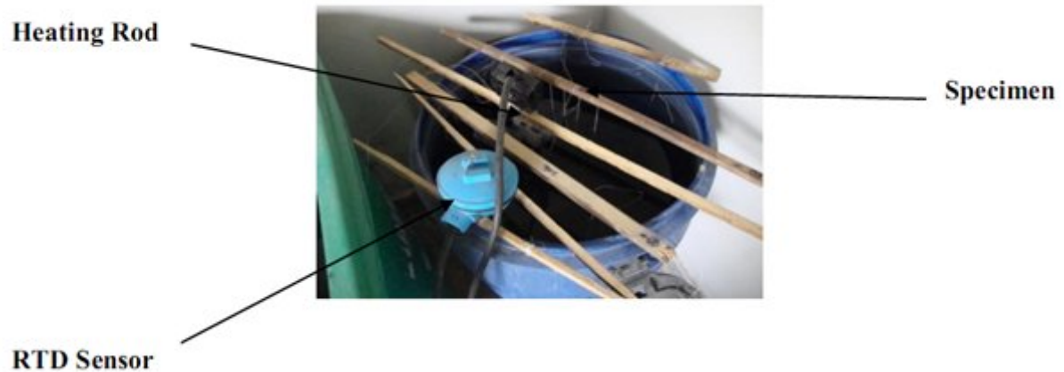
Fig. 4.11 Heating element and RTD sensor in a tank
