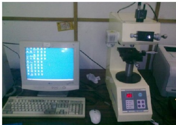
Fig. 4.18 Micro hardness equipment
