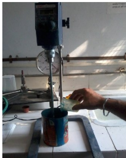
Fig. 4.6 Mixing of hardener to the base component
