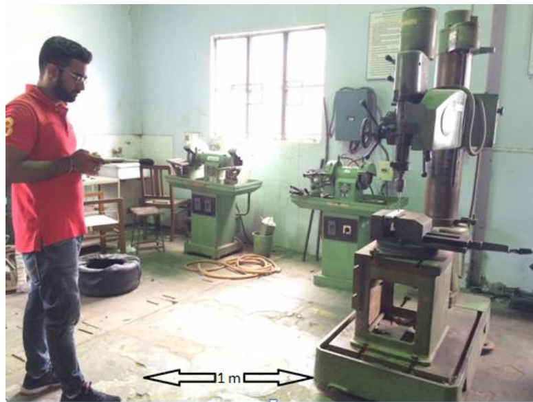
Figure 5.6: Sound pressure level measurement
