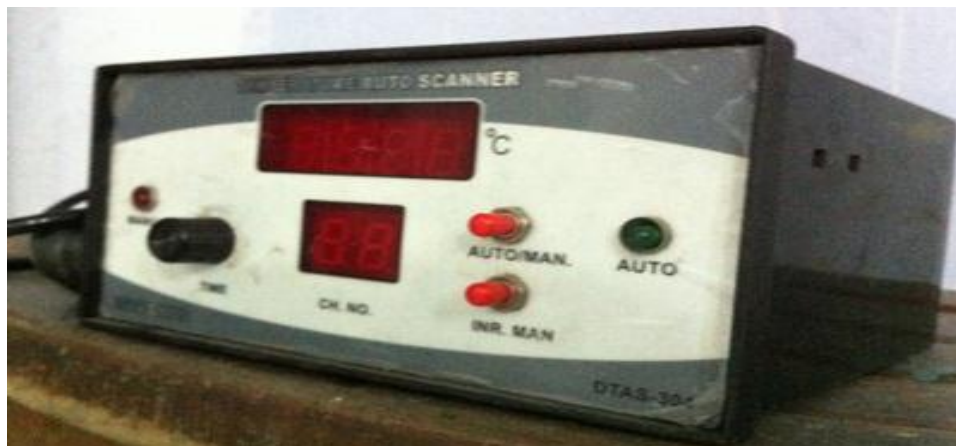
Figure 3.8: Temperature Auto Scanner
