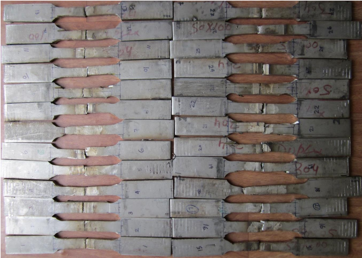
Figure 4.1: Specimen after tensile strength of joints between AISI 304 and Duplex 2205
