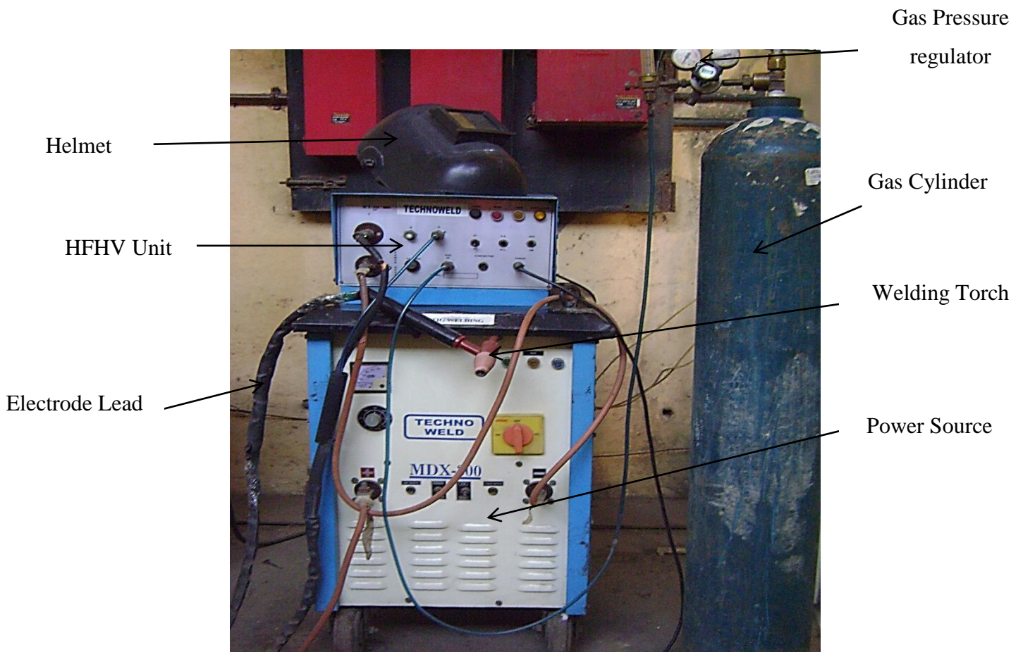
Figure 1.2: Gas tungsten arc welding operation [ http://www.burnsstainless.com ]
