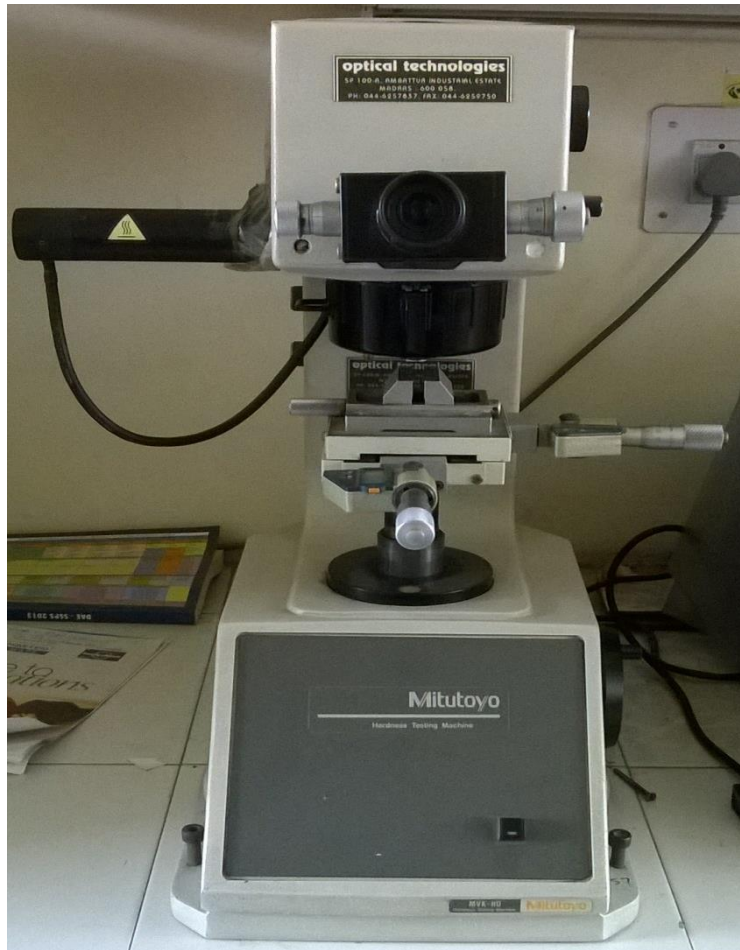
Figure 3.12: Microhardness test machine (Courtesy: School of Physics and Material Science, Thapar University, Patiala)
