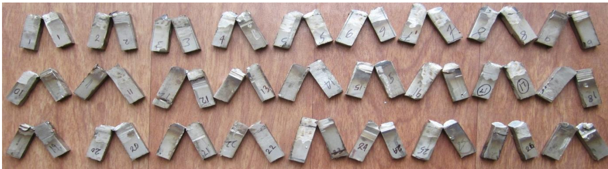
Figure 4.7: Specimens of AISI 304 and Duplex 2205 after toughness test
