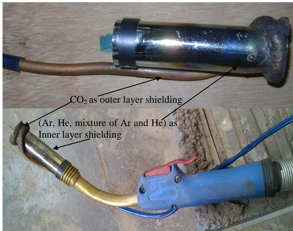
Figure 3.2: Double shielding gas nozzle
