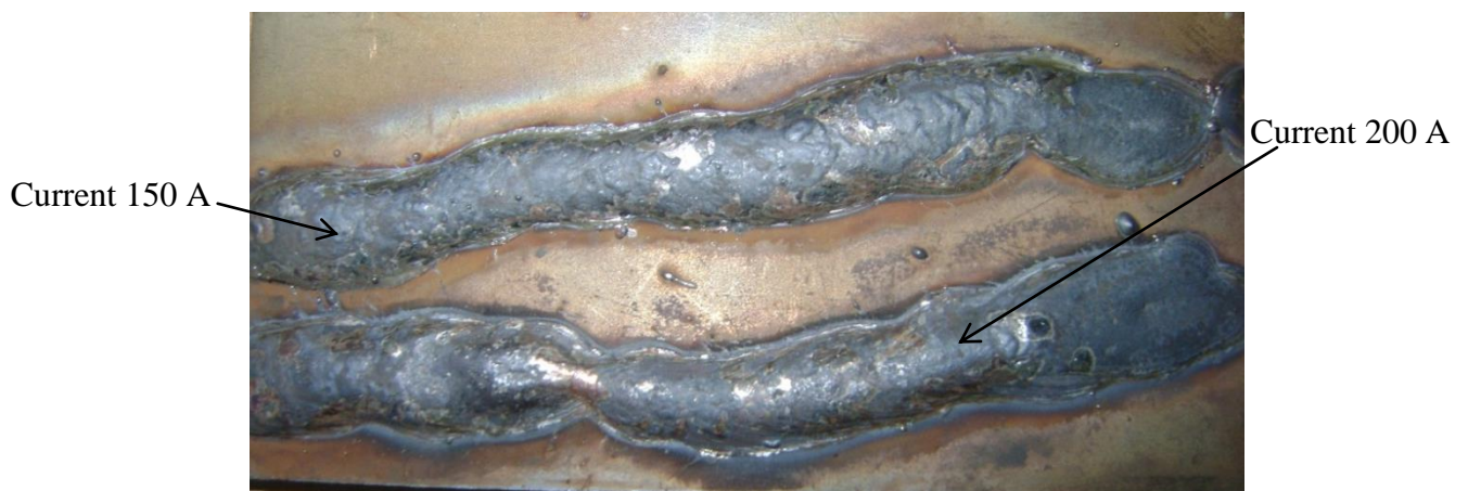
Figure 3.5: Pilot work on Duplex 2205 at different current
