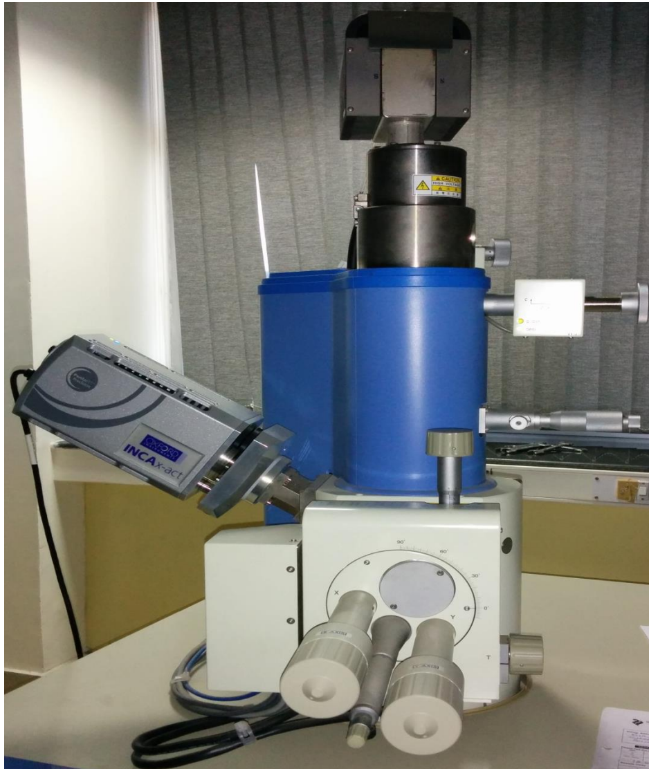
Figure 3.17: Scanning electron microscope (Courtesy: SAI Lab, Thapar University, Patiala)
