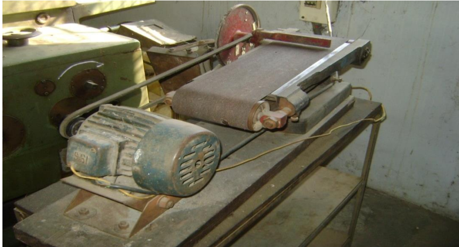
Figure 3.11: Weld grinder (Courtesy: Machine Tool Lab, Thapar University, Patiala)
