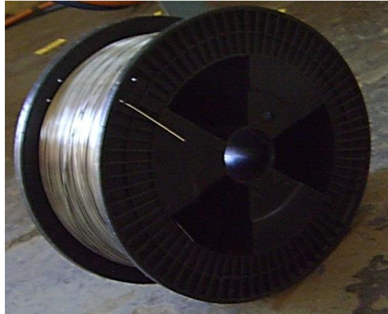
Figure 3.3: ER 304L grade filler wire spool
