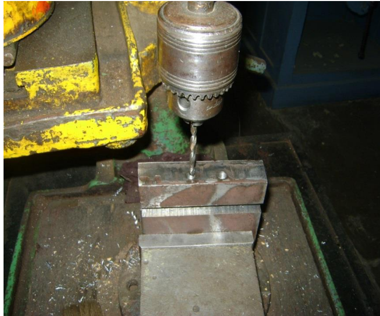
Figure 3.14: Drilling on distortion setup with bench drilling machine (Courtesy: Central Workshop, Thapar University, Patiala)
