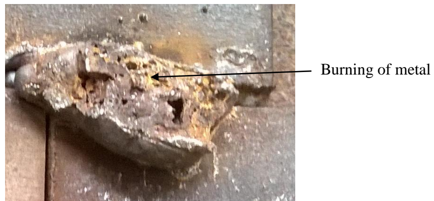
Figure 3.7: Pilot work on mild steel show burning of metal
