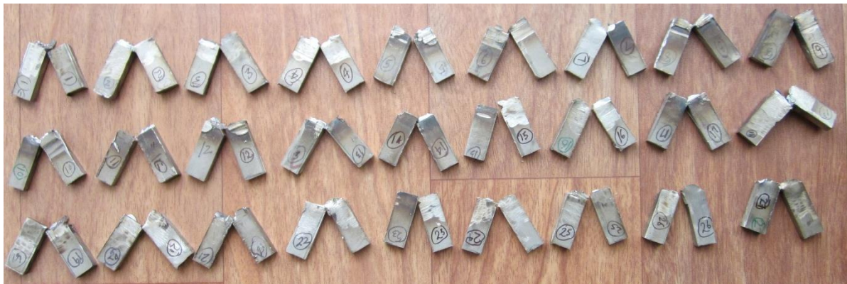
Figure 4.10: Specimens of AISI 304 and Duplex 2205 after toughness test
