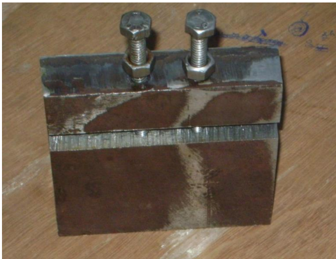
Figure 3.15: Distortion measurement setup
