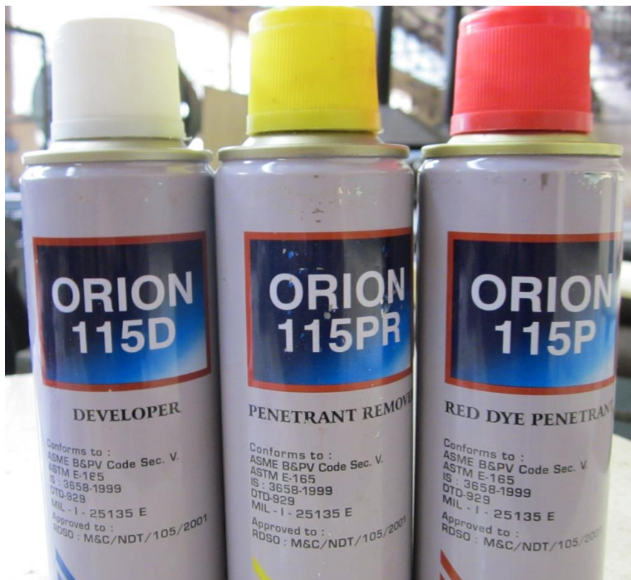
Figure 3.16: Checkmate's cleaner, penetrant & developer used for DPT test of specimens
