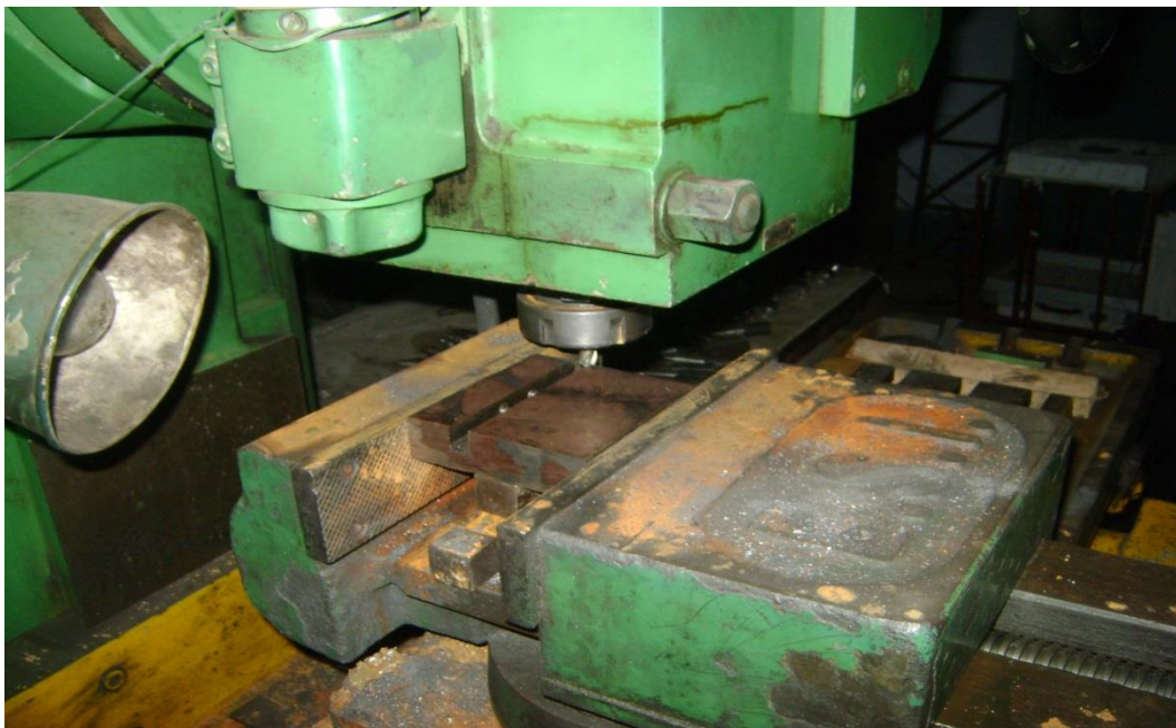
Figure 3.13: Slot cutting on distortion setup with milling machine (Courtesy: Central Workshop, Thapar University, Patiala)
