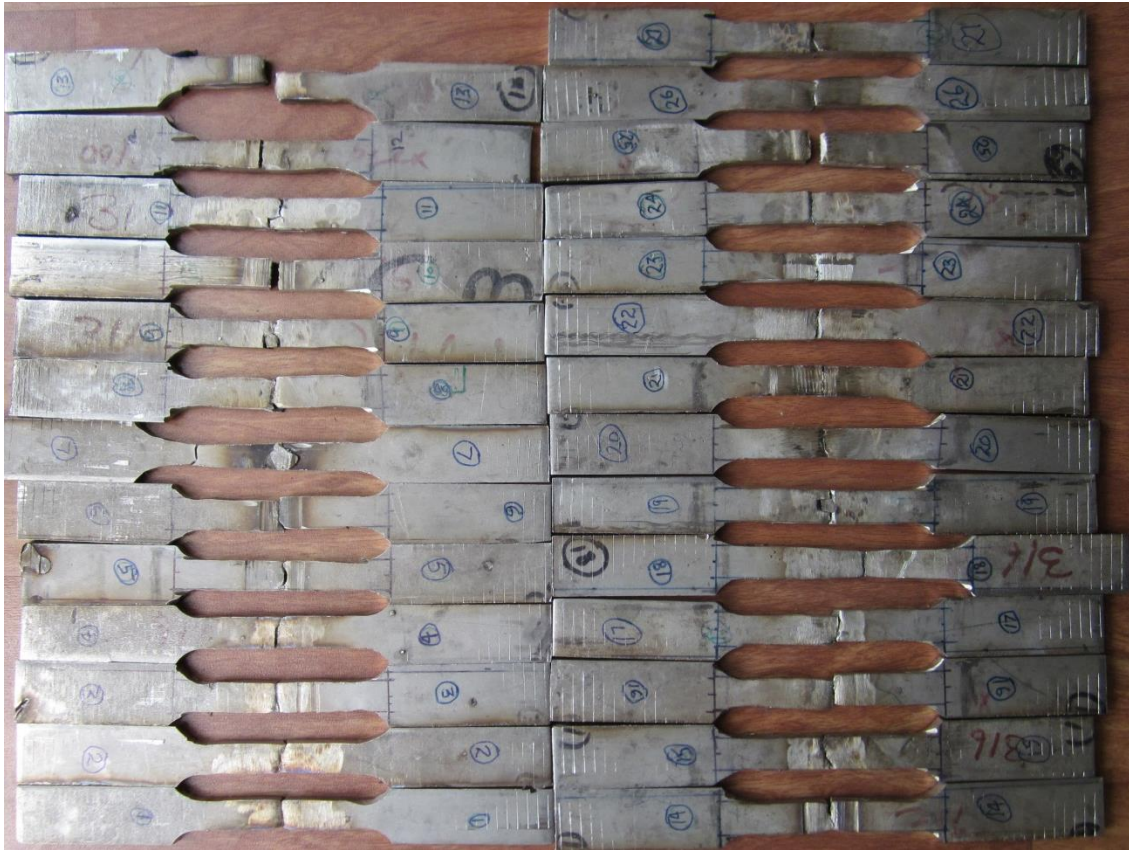
Figure 4.4: Specimen after tensile strength of joints between AISI 316 and Duplex 2205
