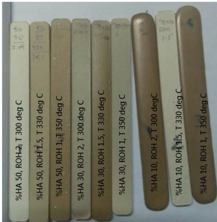
Fig. 4.23 Specimens prepared for delimiting studies
