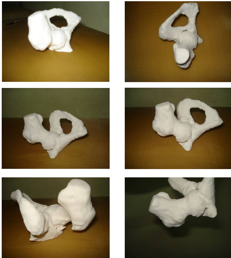
Fig. 4.18 Hip joint prepared through SLS
