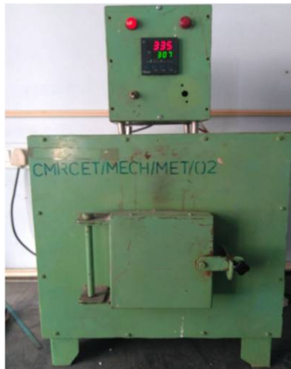
Fig. 4.2 Muffle furnace with programmable temperature controller
