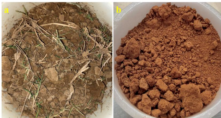
Fig. 2.7 Type of soil used in burying process of films (a) non-sterile soil, and (b) sterile soil
