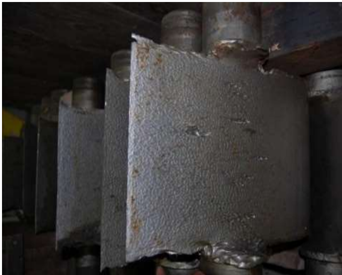
(a) Eroded guide vanes
