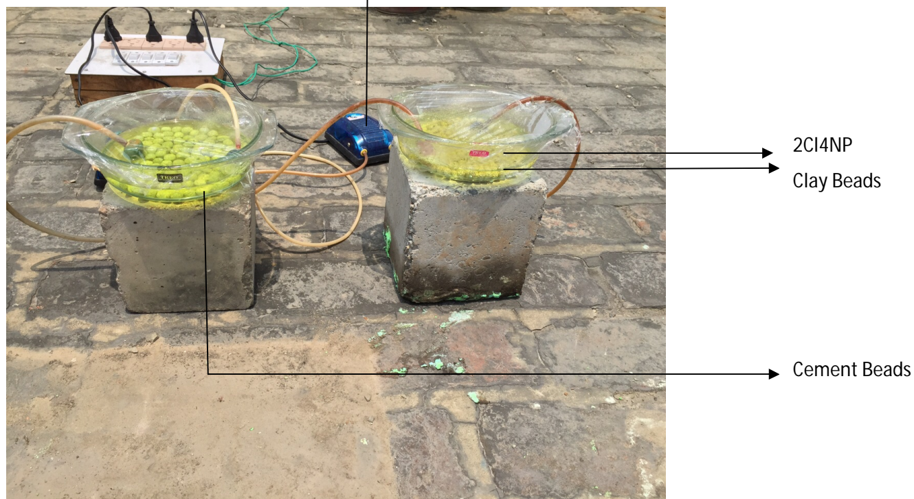
Figure 10: Lab Scale Slurry Reactor ( \text{TiO}_2 immobilized on cement and clay beads) in Sunlight.
