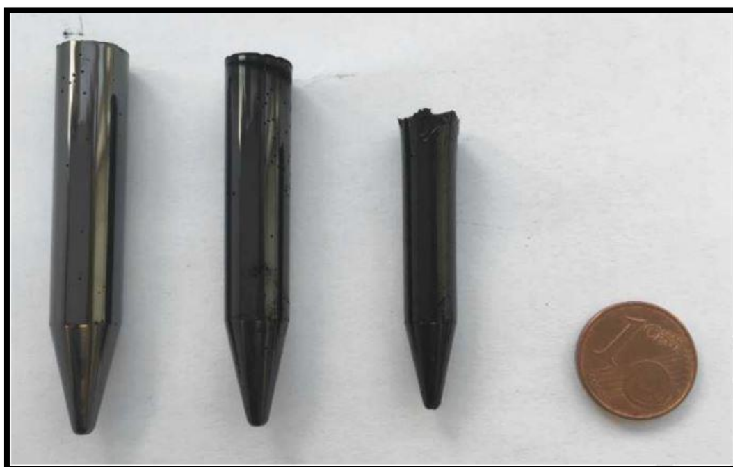
Fig. 2.2 Photograph of the carbon monoliths compared to a one cent coin (reproduced from reference [132])
