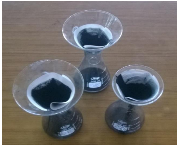
Figure 3.3: filtration of coal after chemical treatment
