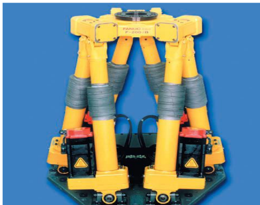
Figure 4.1 Fanuc F-200iB (left) and Face plate (Right)
