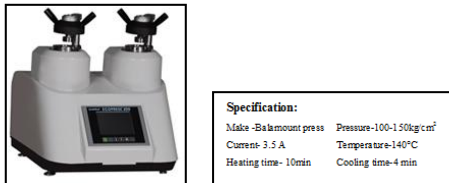
Figure 3.11 Mounting Press with Specification
