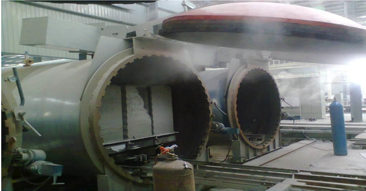
Figure1.5: Steam curing chamber
