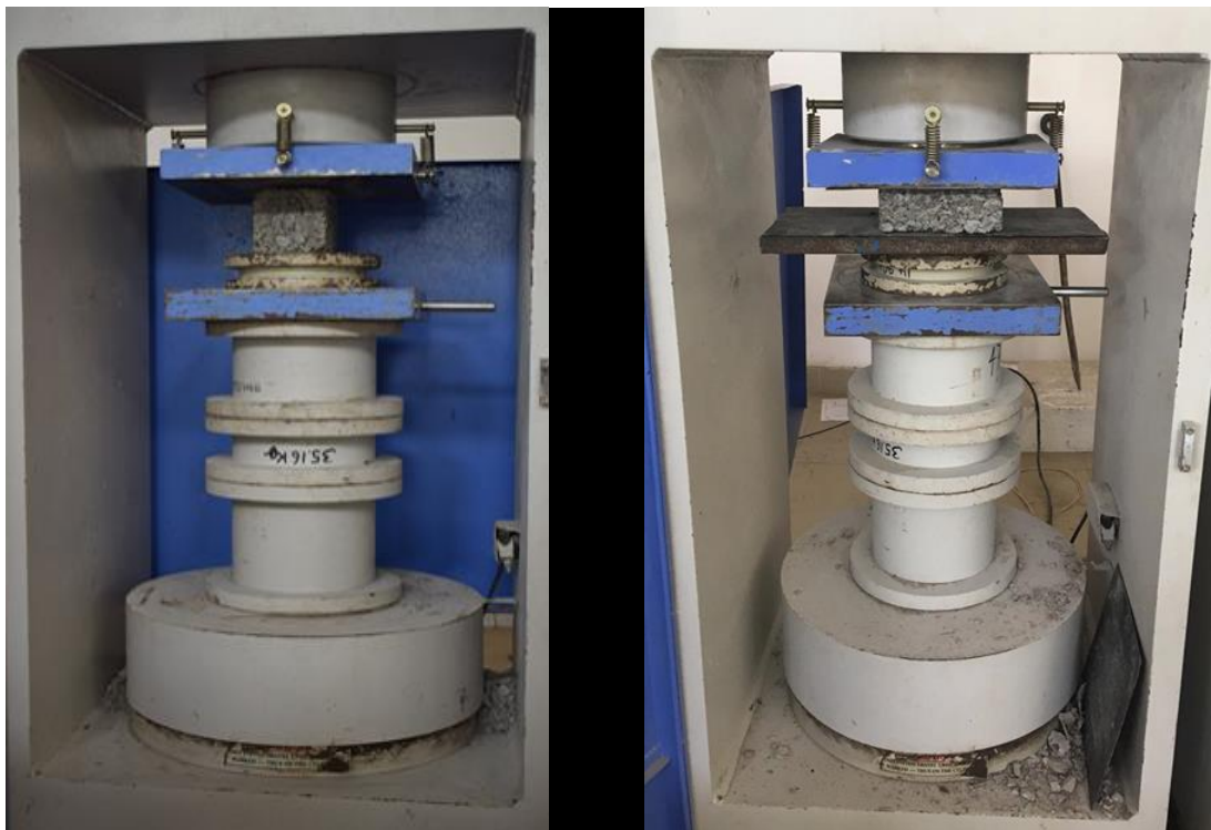
Figure 3.7: Compression testing of cubes and tiles
