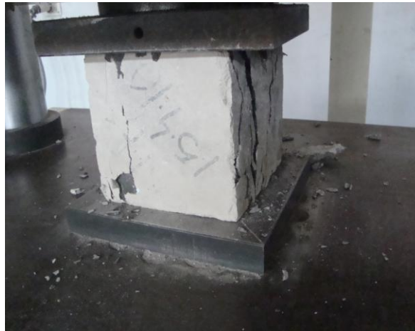
Fig. 3.4: Compression failure of cube without fly ash
