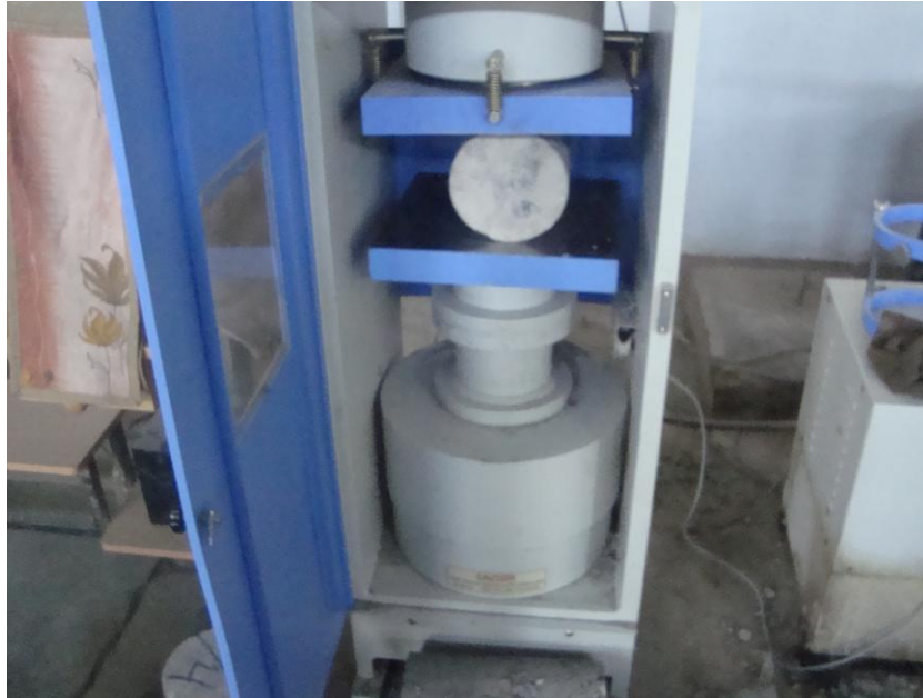
Fig. 3.5: Splitting tensile strength testing machine
