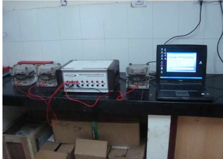
Fig. 3.8: Rapid chloride permeability test set up
