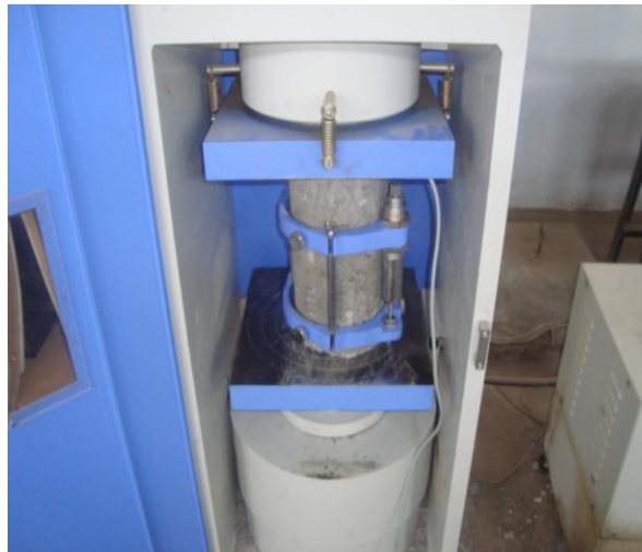
Fig. 3.6: Modulus of elasticity testing machine
