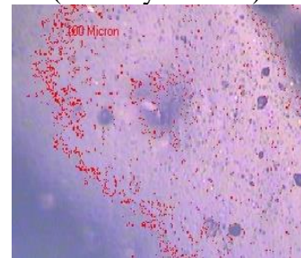
Sample at Serial number 6 (Porosity 9.60%)
