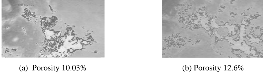
Figure 5.19 Porosity results for (a): Sample 2 and (b) Sample 8 as per Table 4.3
