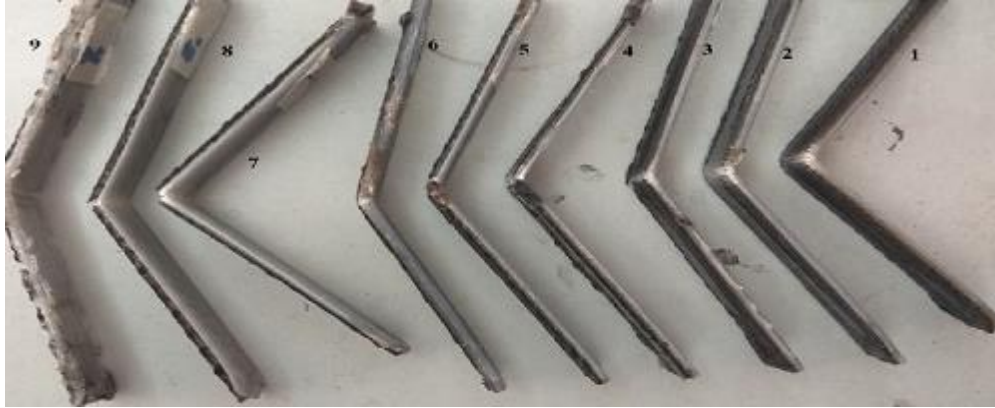
Figure 5.74 3D printed flexural specimens (a) Top view, (b) bottom view, and (c) UTM tested flexural specimens as per Table 4.8
