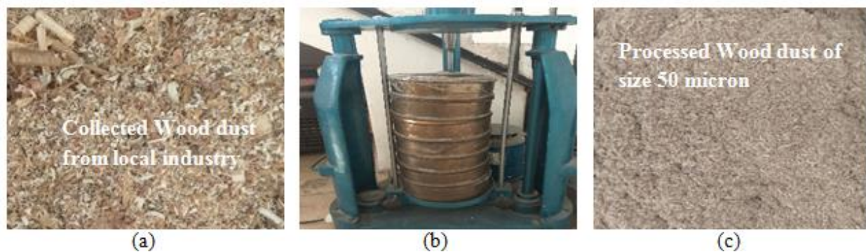
Figure 4.1 processing of wood dust (a) collection, (b) sieve shaker machine, and (c) fine wood particle (50 microns)
