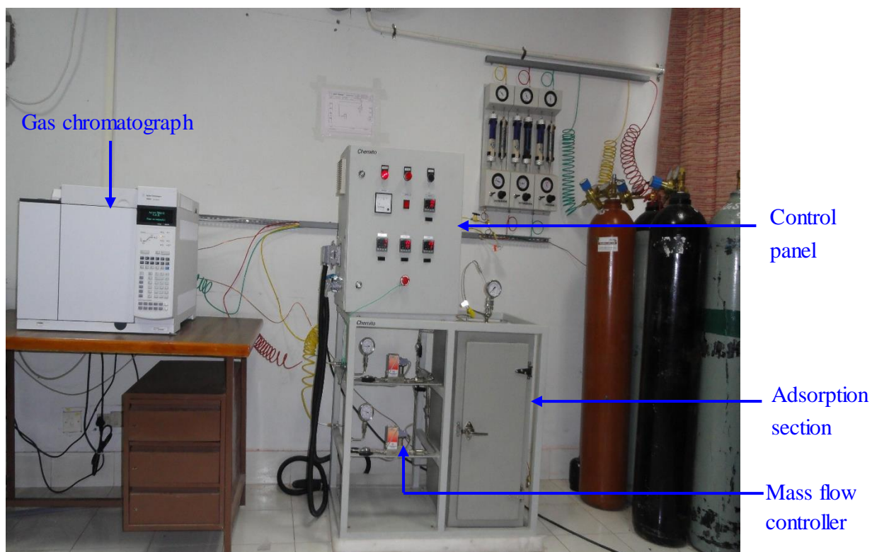
Figure 3.2 Adsorption study set up coupled with gas chromatograph
