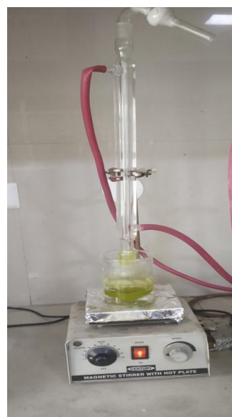
Figure 3.3: Reaction set up for the Ni complex synthesis
