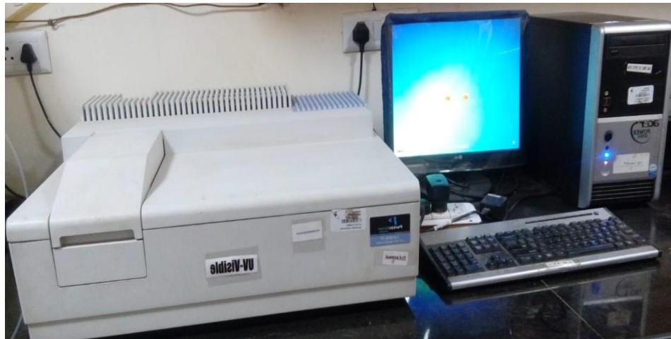
Figure 3.5: Set up for the UV – Visible Spectroscopy
