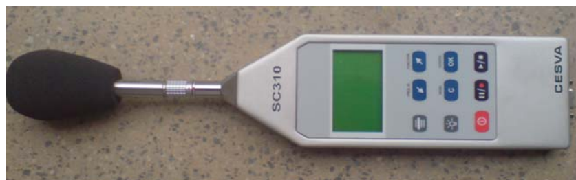
Fig 1.6 Sound level meter with windscreen
