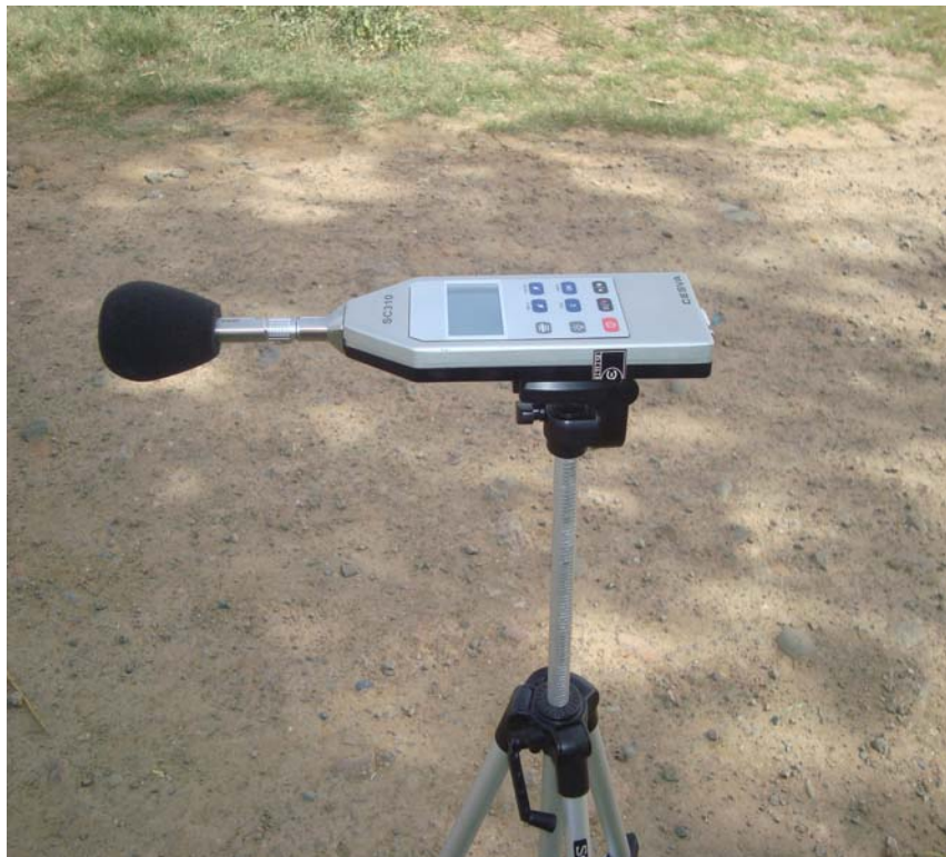
Fig. 4.2 Sound level meter on a tripod with windscreen
