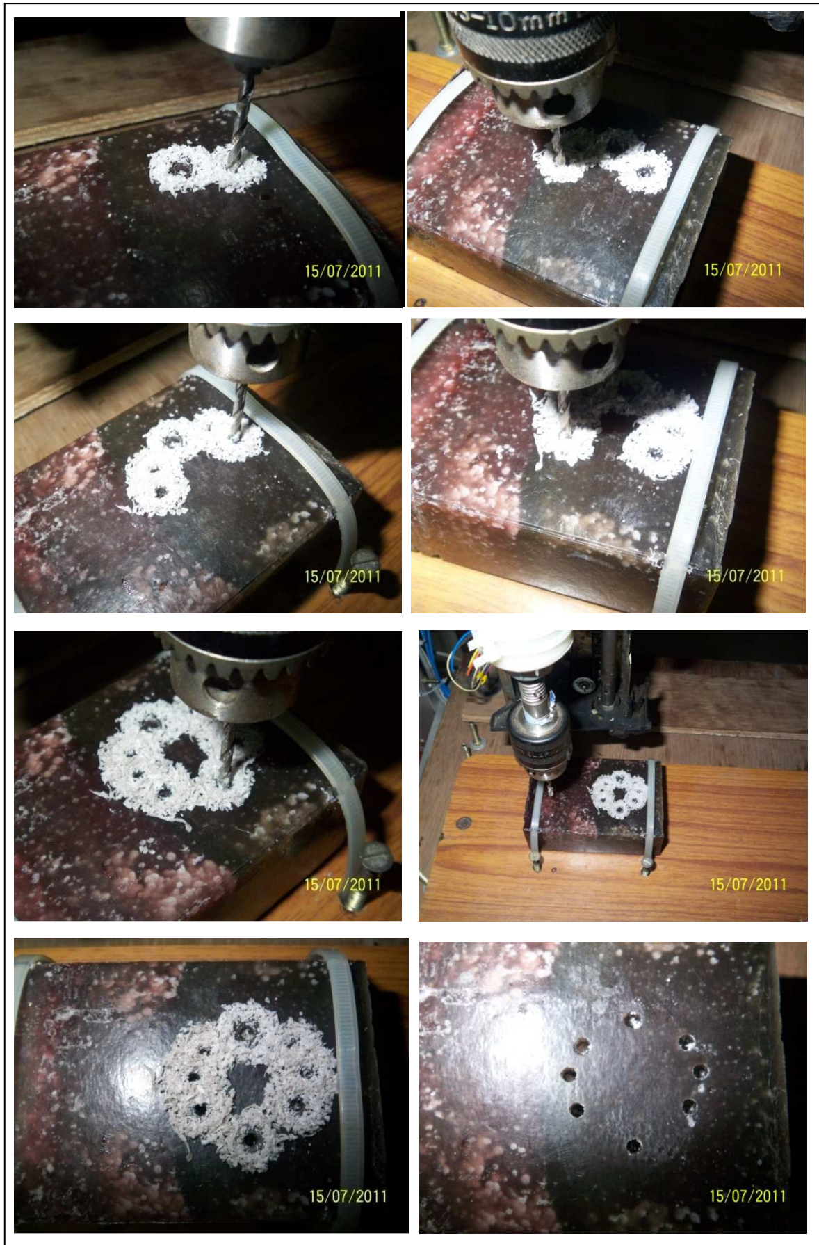
Figure 7.6: Sequence of Cutting on Wax Brick According To Tool Path File Loaded.
