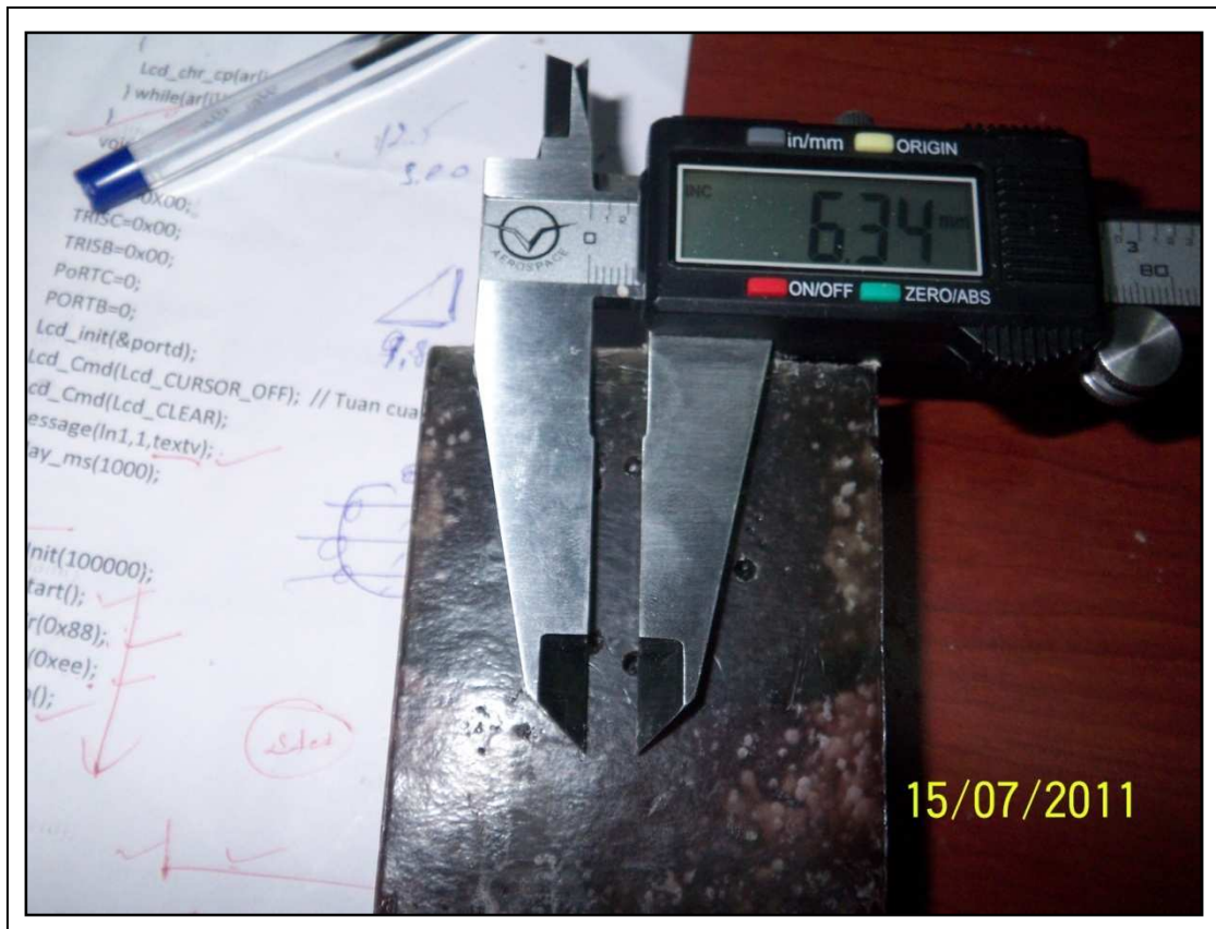
Figure 7.9: Distance Measured of a Point Lie in First Quadrant from Horizontal Diameter of Circle.
