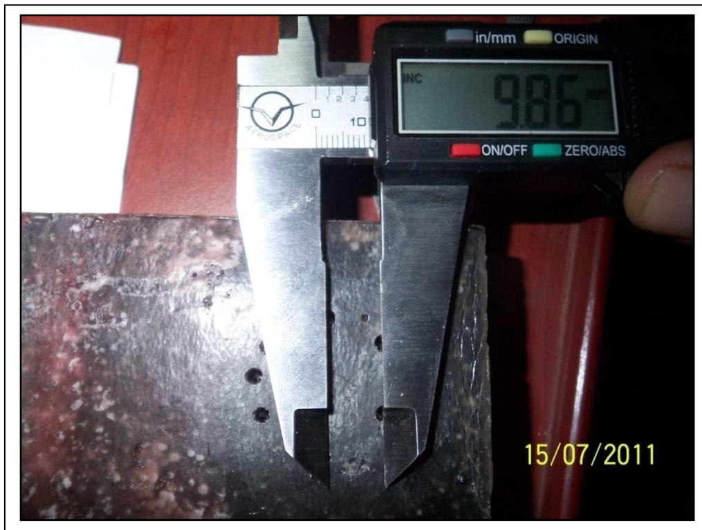
Figure 7.8: Distance Measured of a Point Lie in First Quadrant from Vertical Center Line of Circle.
