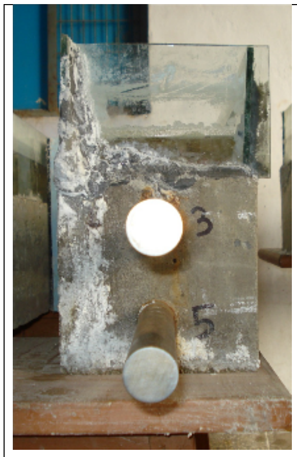
Fig 3.1: Beam specimen with a glass pond (5%NaCl)
