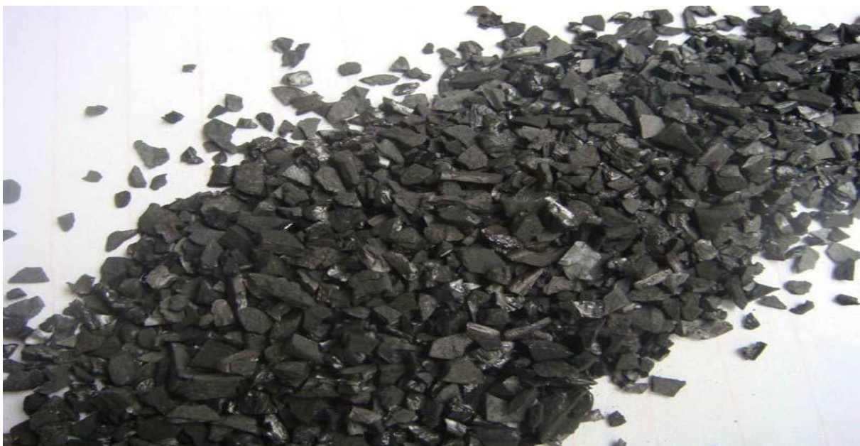
Fig.1.3 Granular Activated Carbon
