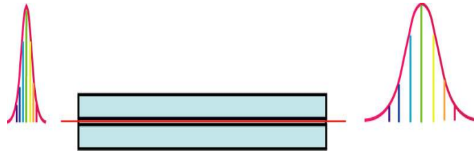
Fig.3.2. Pulse broadening due to chromatic dispersion [37]
