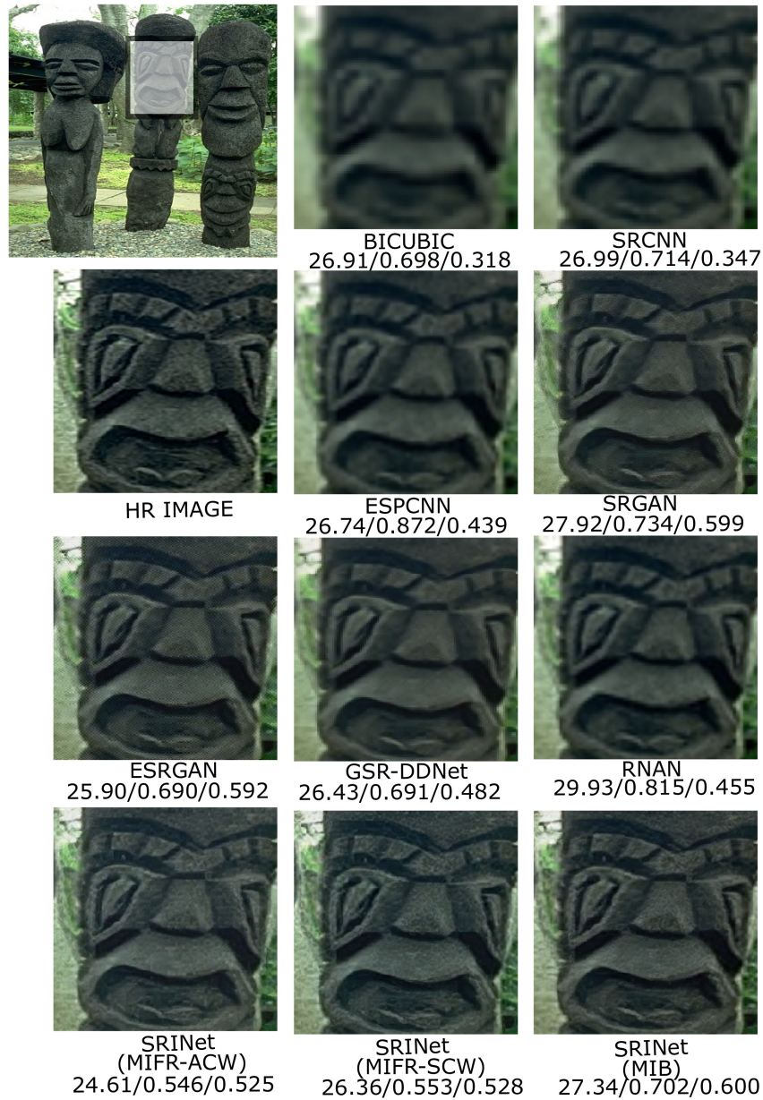
Figure 5.10: Perceptual results with their PSNR/SSIM/VIF score on the '101085' image from the BSD100; upscaled by \times 4 factor.
