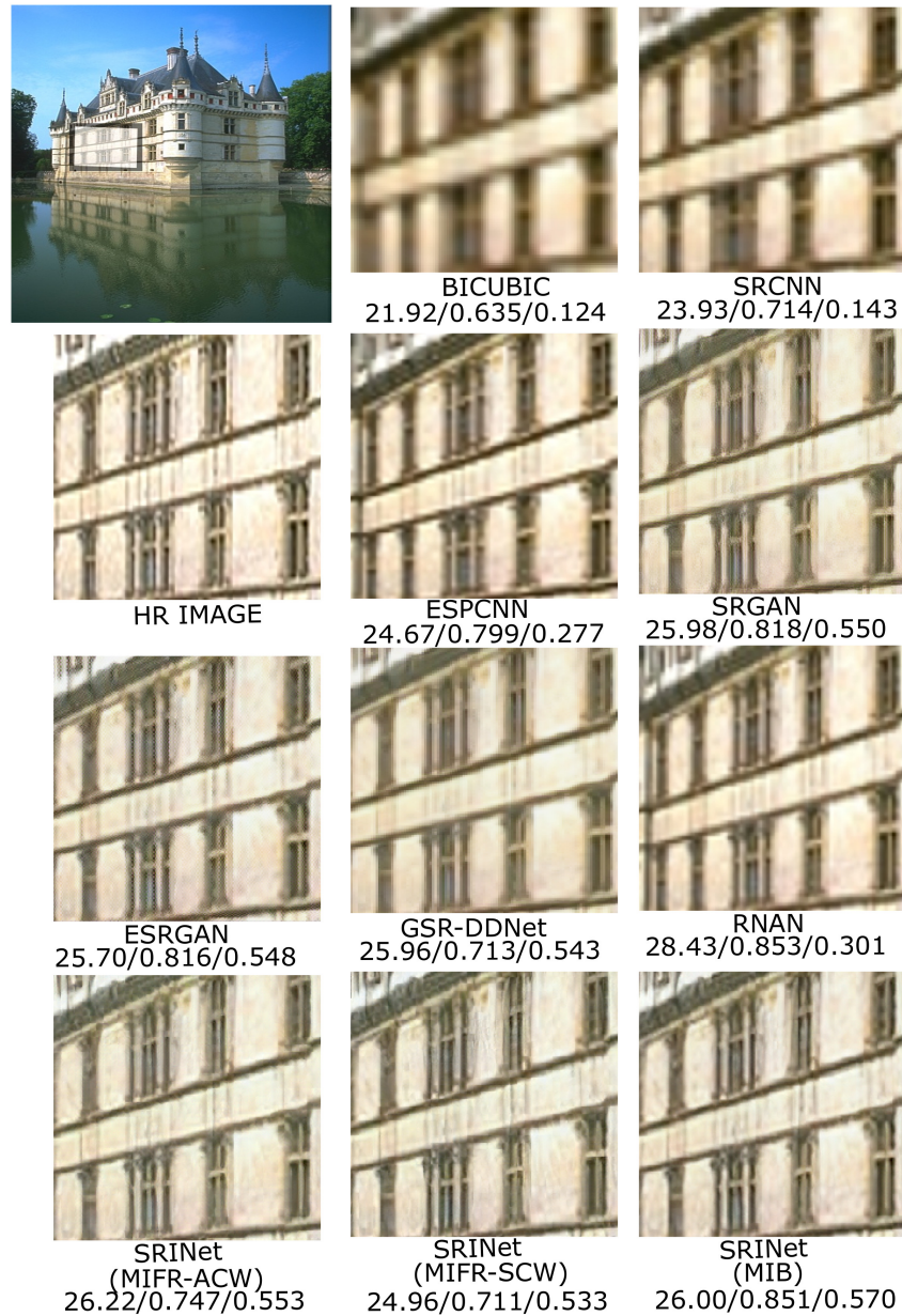
Figure 5.11: Perceptual results with their PSNR/SSIM/VIF score on the '102061' image from the BSD100 test dataset; upscaled by \times 4 factor.
