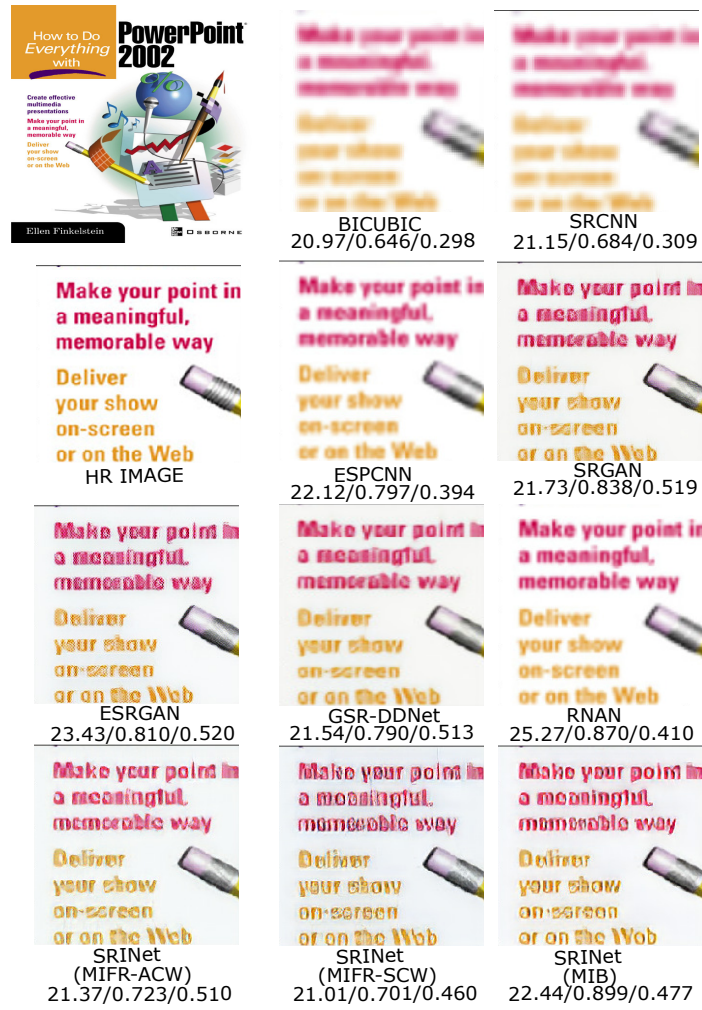
Figure 5.8: Perceptual results with their PSNR/SSIM/VIF score on the ‘ppt3’ image from the SET14; upscaled by \times 4 factor.
