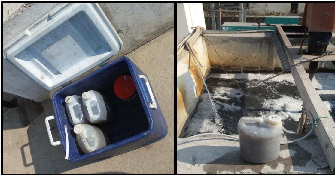
Figure 3-25 Sampling of Wastewater in 2Ltr Plastic Bottle
