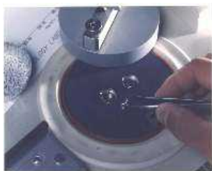
Fig 4.2 Sample holder of DSC
