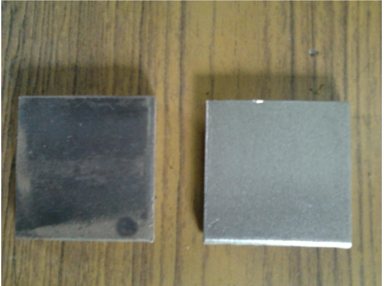
Fig. 1.2 Mild Steel (99.0% Fe, 0.101%C, 0.173% Si, 0.532% Mn ) work piece before and after 15 minutes of steel shot blasting)
