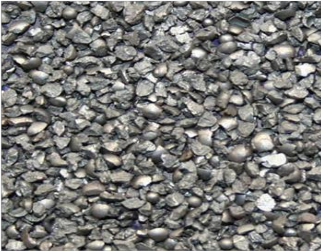
Fig. 1.6 Chilled iron grit
