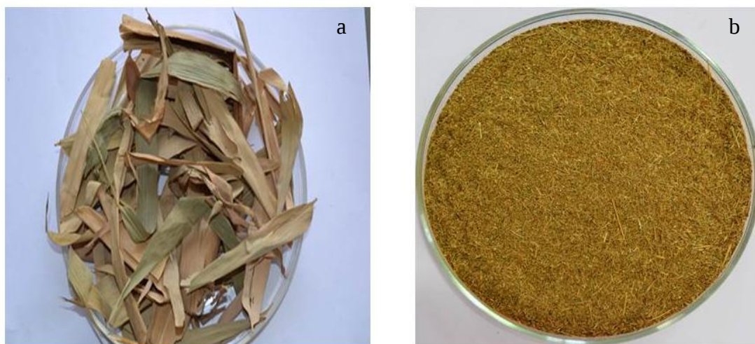
Figure 7. a. Washed and dried Bamboo leaf litter (BLL); b: Pulverised BLL (0.5 mm).
