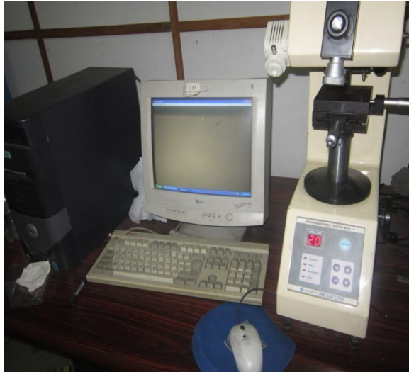
Figure 3.12: Micro hardness testing machine Model: MVH2 (Courtesy: Advance Measurement Lab, Thapar university, Patiala)
