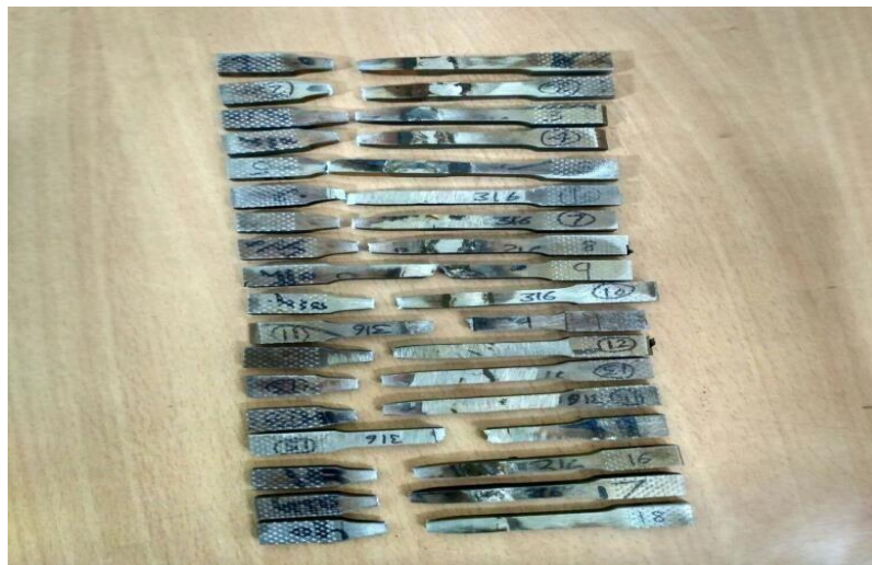
Figure 4.1: Broken specimen from tensile test
