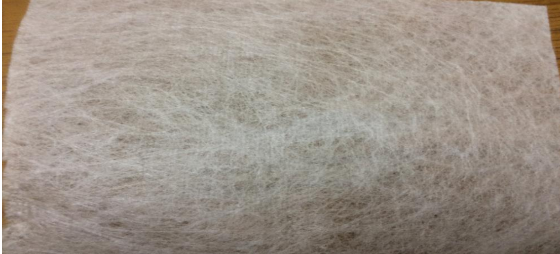
Figure 1.3: Pictorial representation of non-woven geotextile.
