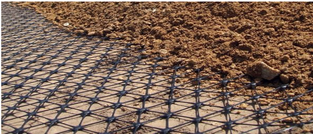
Figure 1.5: Pictorial representation of geogrid ( www.tensarcorp.com ).
