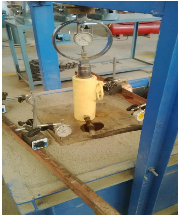
Figure 3.5: Loading and Strain measurement used in the test.
