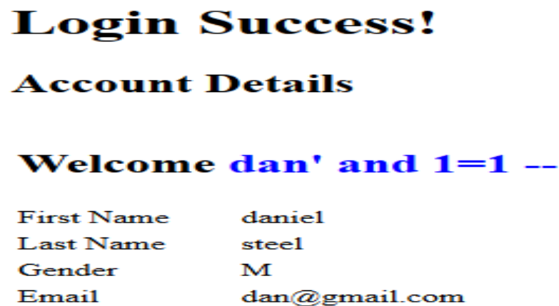
Fig. 4.10: Blind Injection Attack part (b)
