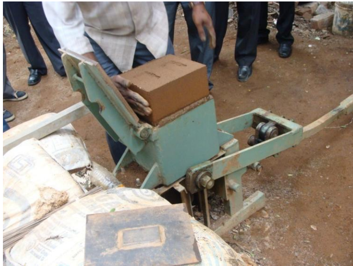
Fig. 4.4.20. Set up for making soil cement blocks (Reddy and Jagadish, 2003)
