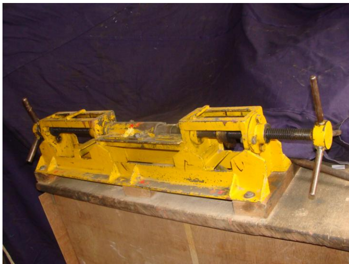
Fig. 3.1. Apparatus for preparing sand columns
