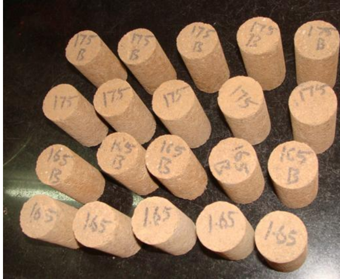
Fig. 4.4.13. Preparation of varying density sand columns by block making machine
