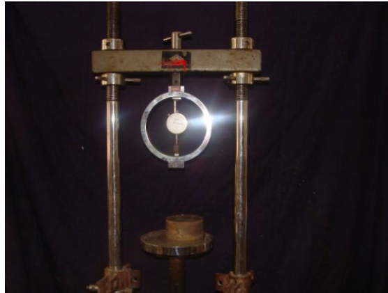
Fig. 4.4.15. Machine showing set up for measurement of Compressive strength
