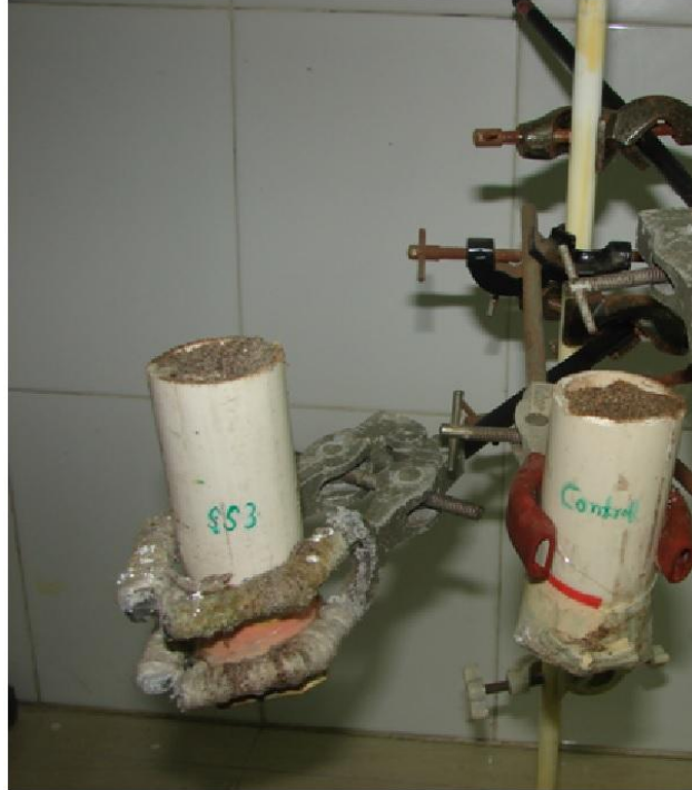
Fig. 4.4.1. Assembly of microbial sand columns
