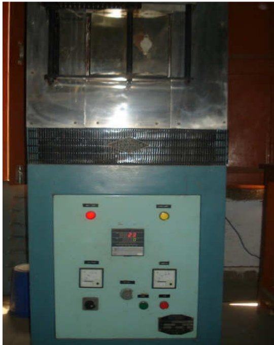
Figure 2.6 Programmable high temperature furnace for sintering with its specification
