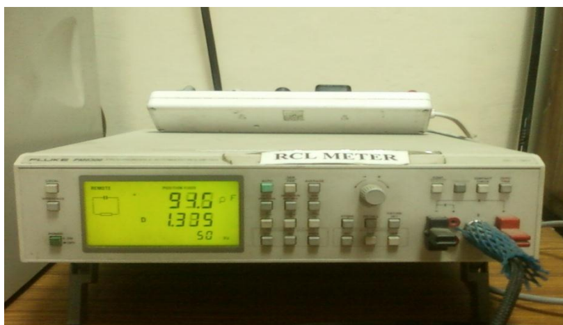
Figure. 2.5 Programmable automatic RCL meter [FLUKE PM6306] used for dielectric studies.
