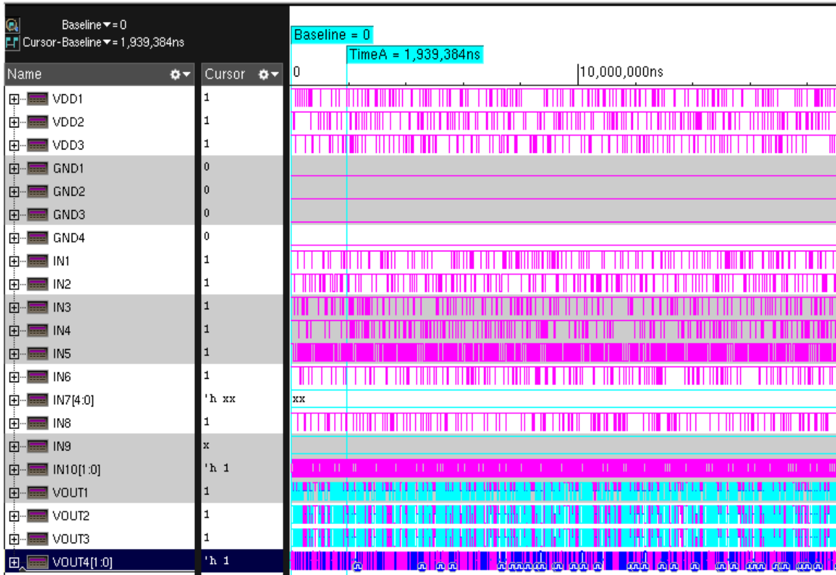
Figure 7.23 Simulation result of Voltage Regulator Model with all valid random sequence
