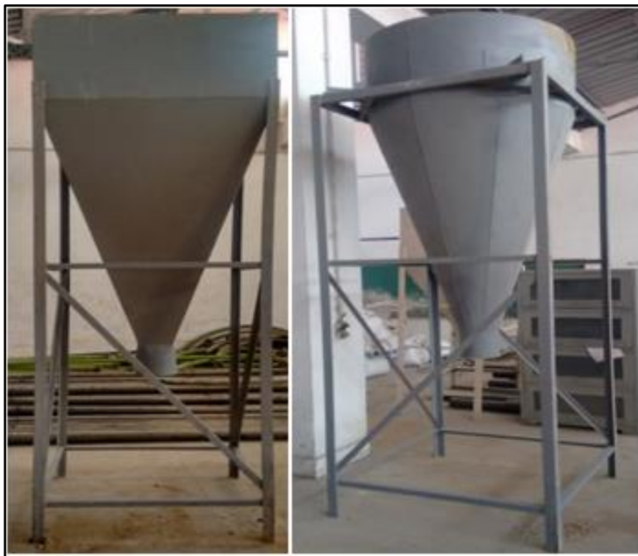
Figure 4.11: Picture of fabricated trapezoidal (left) and conical (right) hoppers
