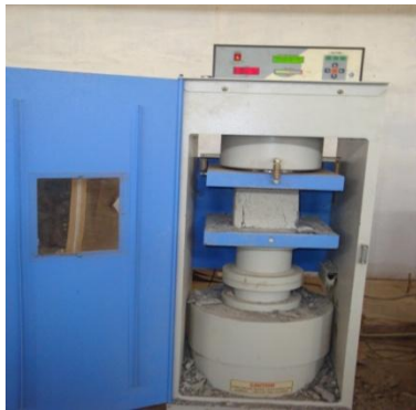
Figure 3.10 Compressive strength measurements (ACTM) (Structure lab TU, Patiala)
