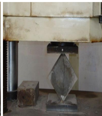
Figure 3.11 Splitting tensile strength measurements (UTM) (Structure lab TU, Patiala)
