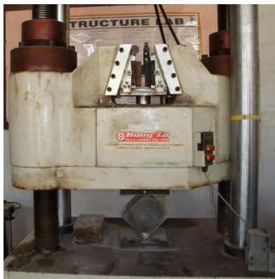
Figure 3.11 Splitting tensile strength measurements (UTM) (Structure lab TU, Patiala)
