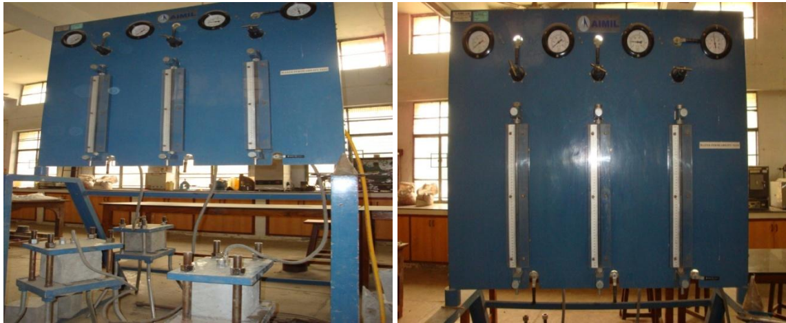
Figure 3.12 Depth of water penetration measurements (WPTM) (from Structure lab TU, Patiala)
