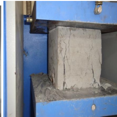
Figure 3.10 Compressive strength measurements (ACTM) (Structure lab TU, Patiala)
