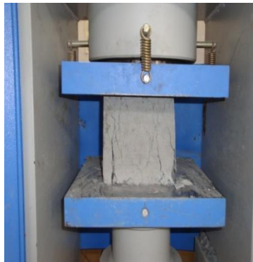
Figure 3.10 Compressive strength measurements (ACTM) (Structure lab TU, Patiala)
