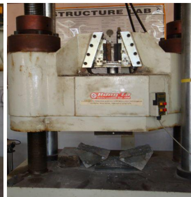
Figure 3.11 Splitting tensile strength measurements (UTM) (Structure lab TU, Patiala)
