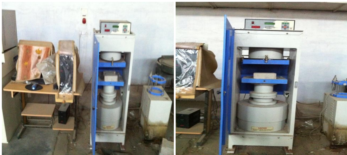
Figure 3.2 Automatic compressions testing machine (courtesy: Structure lab TU, Patiala)
