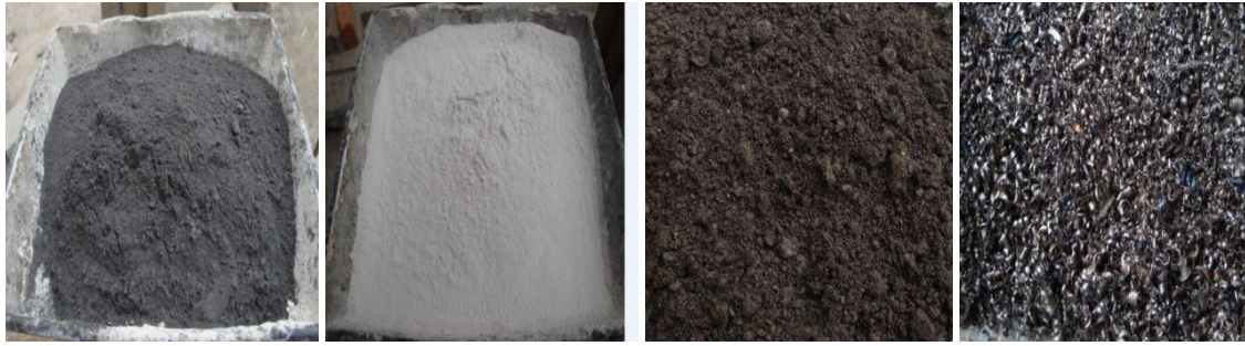
a) Electric arc furnace slag (b) Glass powder (c) Steel powder (d) steel scrap
