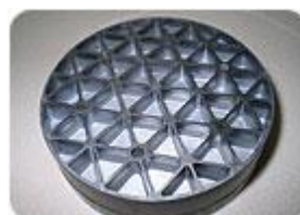
Fig. 1.12:- Honeycomb structure machined on the back of a silicon mirror [49]
