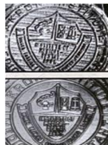
Fig 1.14:- Coin with grooving carried out with USM [49]
