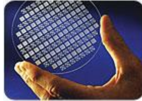
Fig. 1.10:- Square cavities, round through holes and crossing beams in a 4-in borosilicate wafer [49].
