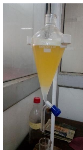
Figure 3.4: SOME after water wash
