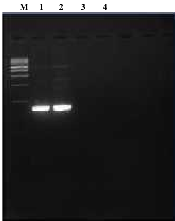
Figure 5.8: Comparison the effect of gold and Al 2 O 3 nanoparticles on PCR. Lane M is for marker; Lane 1 is for control without gold nanoparticles; Lane 2 having 0.5% of 30nm gold nanoparticles; Lane 3 having 0.5% of 40nm Al 2 O 3 ; Lane 4 having 0.5% of gold and Al 2 O 3 in combination.
