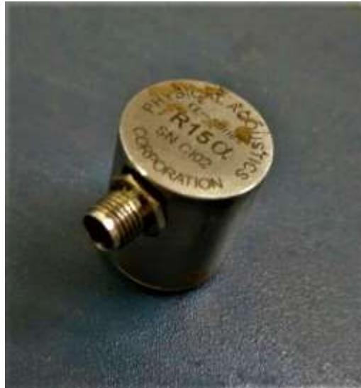
Figure 3.4: R15 \alpha sensor used for mild steel
