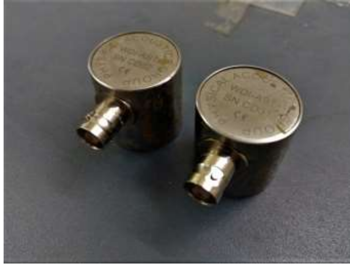
Figure 3.6: WDI-AST sensors used for composite material
