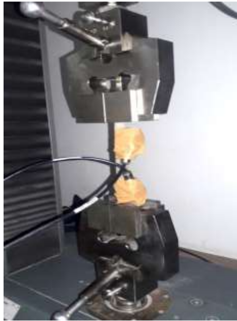
Figure 3.13: Composite Specimen during tensile testing with sensors
