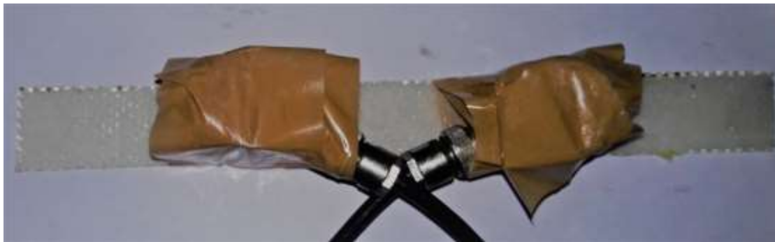
Figure 3.14: AE sensors attached with composite specimen
