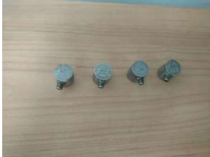
Figure 3.5: R3 \alpha Sensor used for Concrete
