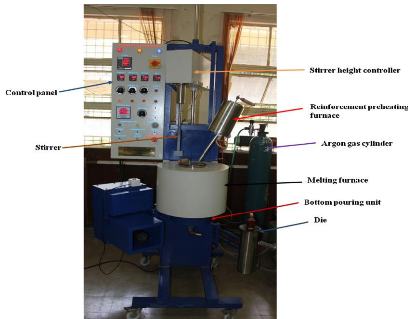
Figure 2.1: Modified stir casting machine setup [12]
