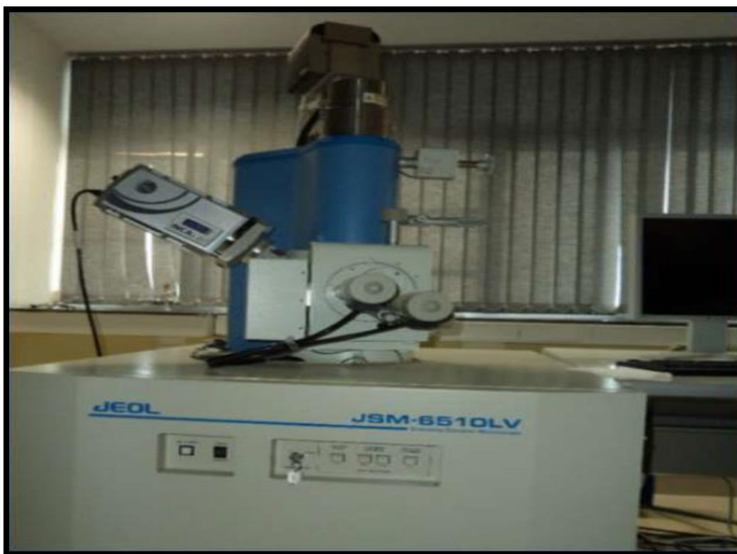
Figure 4.6 Scanning electron microscopy (Make: JEOL JSM -6510LV, Oxford instruments) (Photo courtesy: SAI Labs, Patiala)
