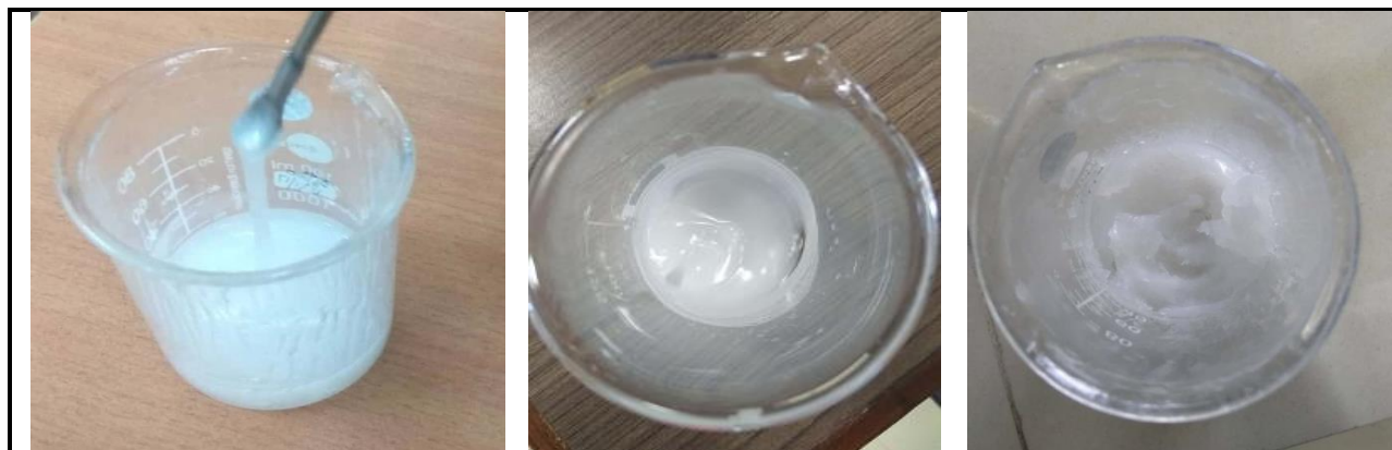
Figure 8.11 STF with 3 phr PEG4600 a) freshly prepared sample (viscous liquid) b) after a week (soft gel) and c) after a month (hard gel)
