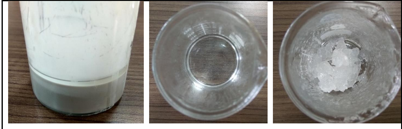
Figure 4.11 STF of a) 60% of 400 nm silica particles b) 20% of 11 nm fumed silica particles and c) 20% of 7 nm fumed silica particles
