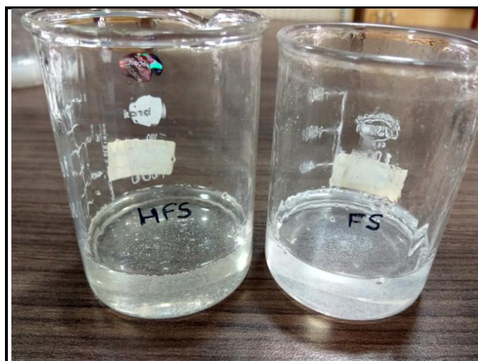
Figure 10.1 STF of a) hydrophobic fumed silica and b) hydrophilic fumed silica dispersed in PPG425
