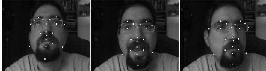
Figure 2.5 The face model constructed by EBGM: (a) an image graph, (b) the facial landmarks of a test image detected by EBGM, (c) the image graph of a test image constructed by EBGM. [25]
