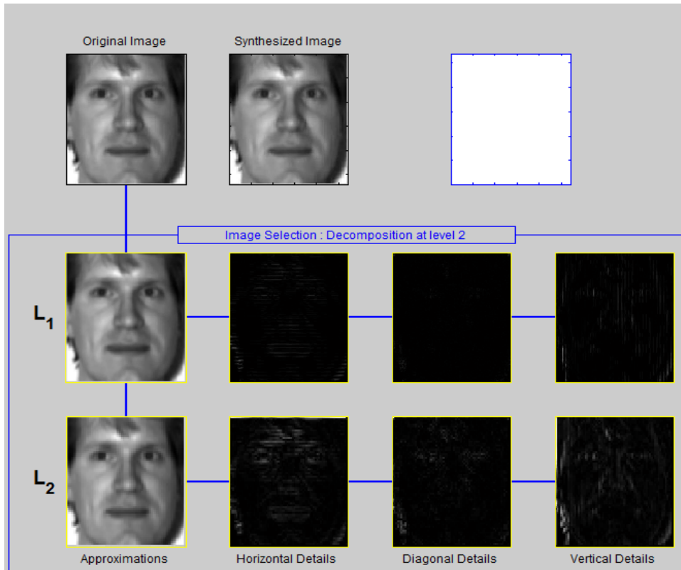
FIGURE 4.11 The decomposition of the Face Image at the HAAR level 2 in TREE mode.
